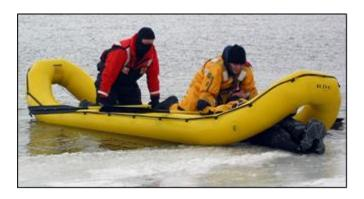
**MARSARS** rescue sled – a sled that can propelled across the ice to a victim. As the sled nears a victim the empty sled becomes a self-rescue reaching device for victims that can assist in own rescue. The sled provides for a quicker extraction by minimizing risk of injury to both victim and rescuer.
