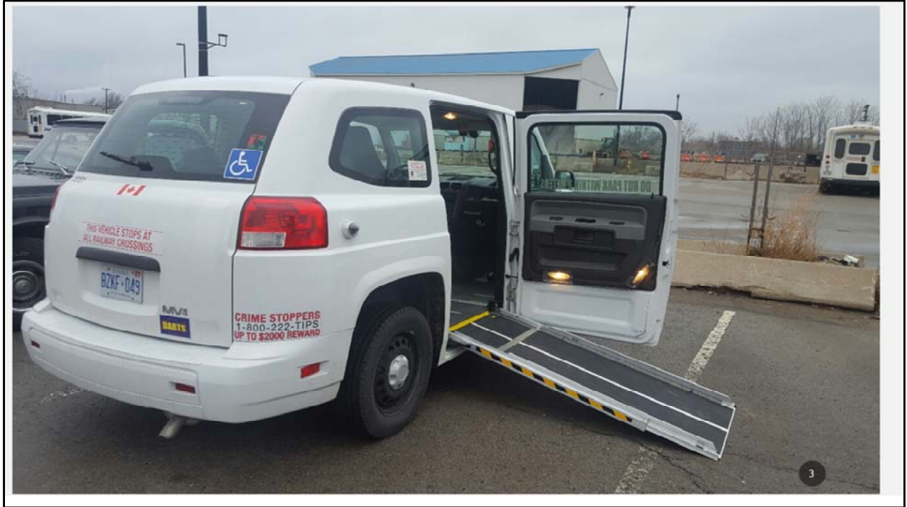
MV-1 with the ramp extended.
