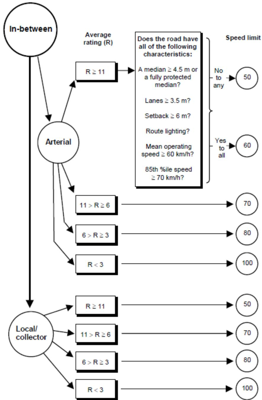
Figure C-3: Speed Limit Flow Chart – In-Between
