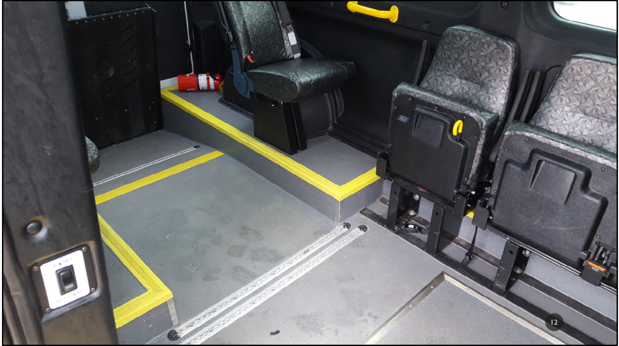
Inside the Promaster showing the floor space for the 2 wheelchairs. Also shows the two seats that are elevated on the back wheel hubs. These are the seats that the travelling public has issue with.
