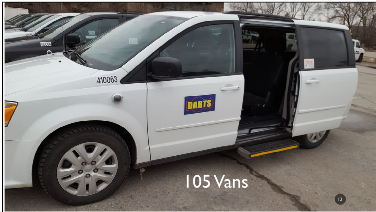
DARTS van showing the installed step (these are on both sides of the vehicle) to assist seniors with entering the van.
