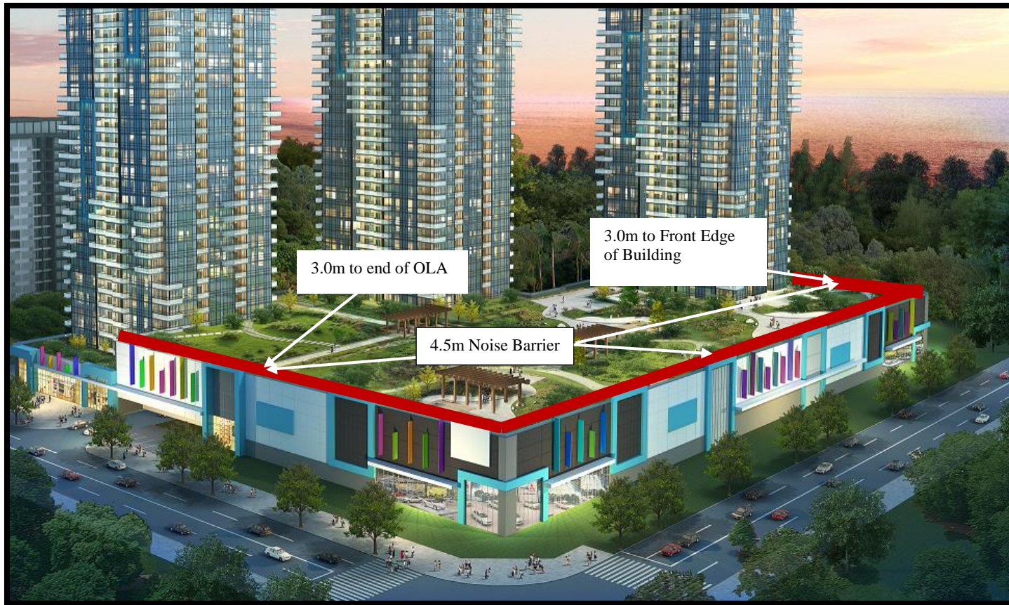
FIGURE 4 NOISE BARRIER LOCATIONS
