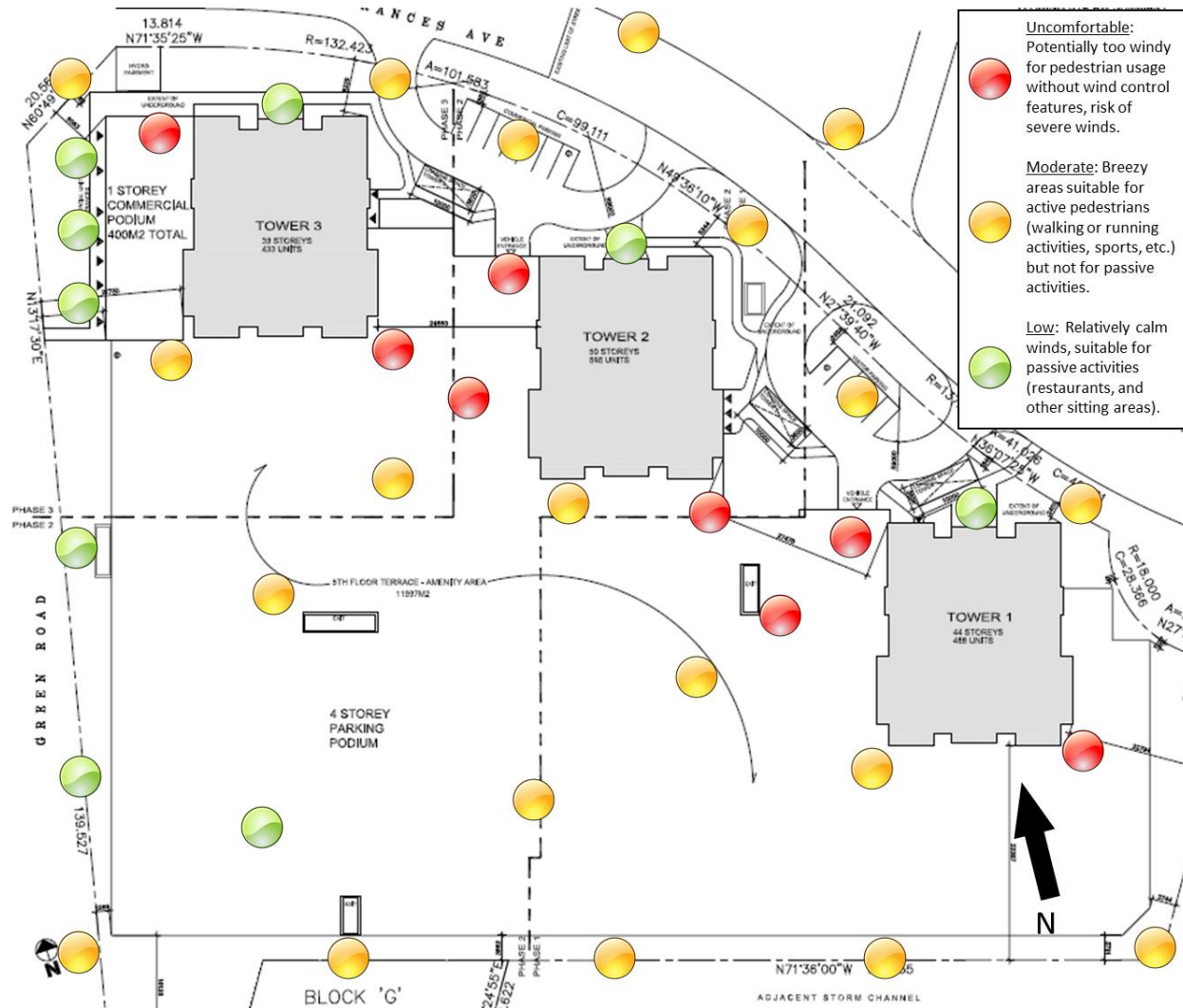
Image 8 – Predicted Relative Winter Wind Speeds at the Base of the Three Towers (Worst Case Condition)
