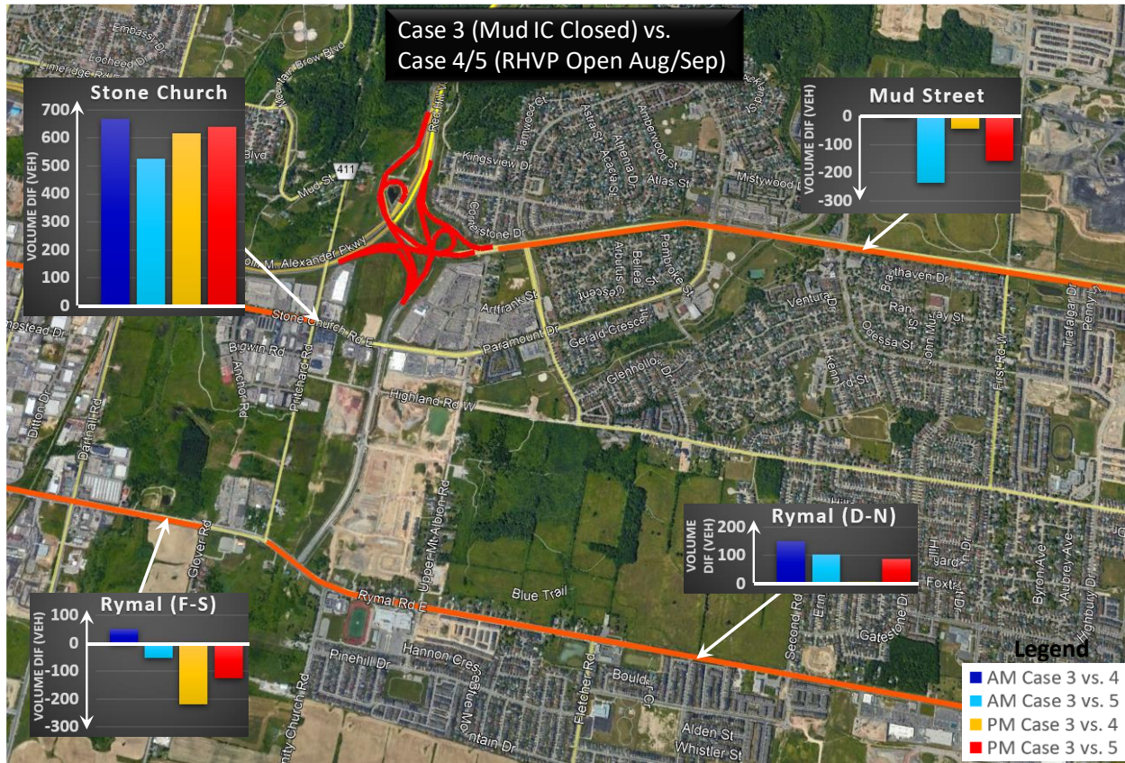
Figure 23: Volume Diversion Comparison: Case 3-Mud IC vs. Case 4-Open Aug and Case 5-Open Sep
