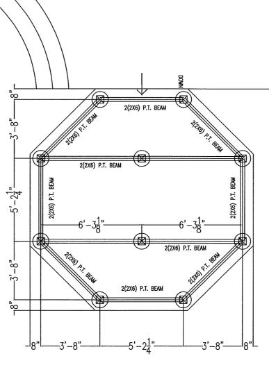
6x6 P.T. POST ON 12" CONCRETE SONOTUBE (4' BELOW GRADE)
