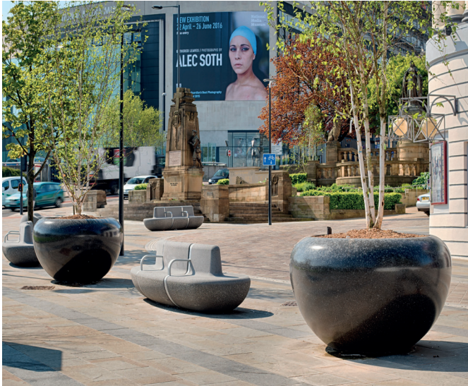
Figure 6: PAS68 rated street furniture, not suitable due to materials, form and scale
