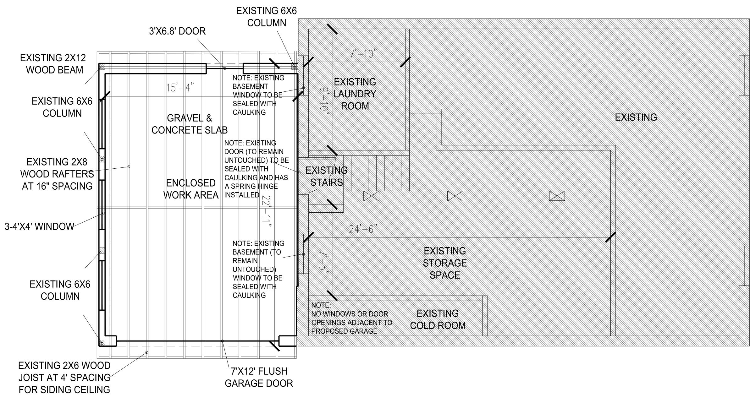
NOTE: EXISTING SIDING CEILING/ ROOF/RAFTERS/JOIST TO REMAIN UNTOUCHED
