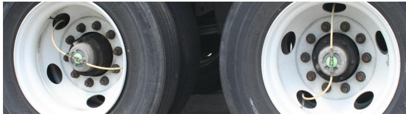
In the U.S., a large truckload carrier with 5,000 tractors and 15,000 trailers averaging 124,000 miles a year on tractors and 41,000 miles on trailers, conducted a fuel economy test with 60 trucks pulling trailers without tire inflation systems and 75 trucks matched with trailers with the systems installed. The results of the test showed a 1.5% improvement in fuel consumption for trucks with ATIS.
