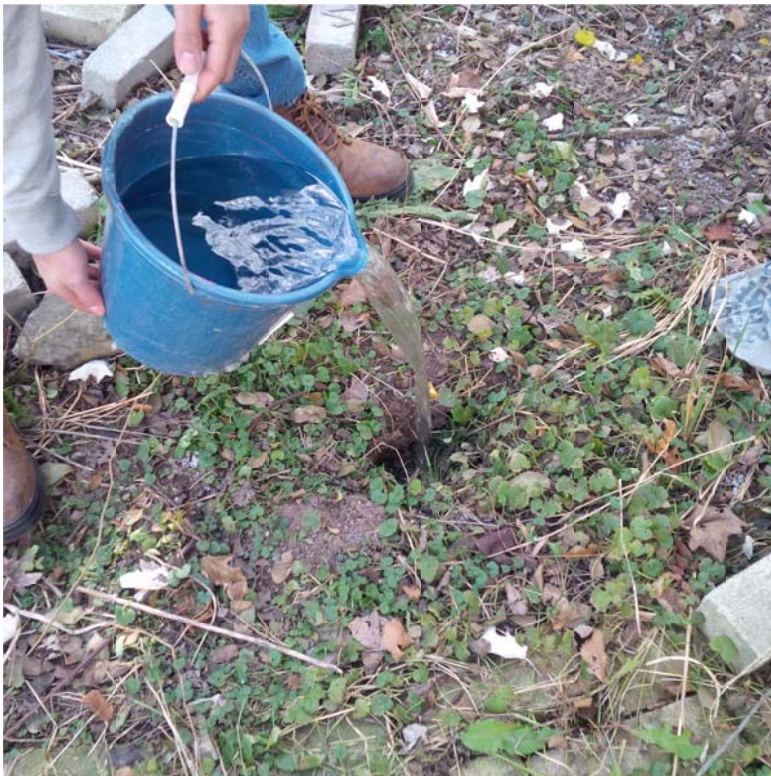
Photograph 8. Impromptu falling head test to observe sinking rate. See report for comments.
