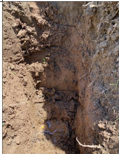
12. Soil profile of existing leaching field
