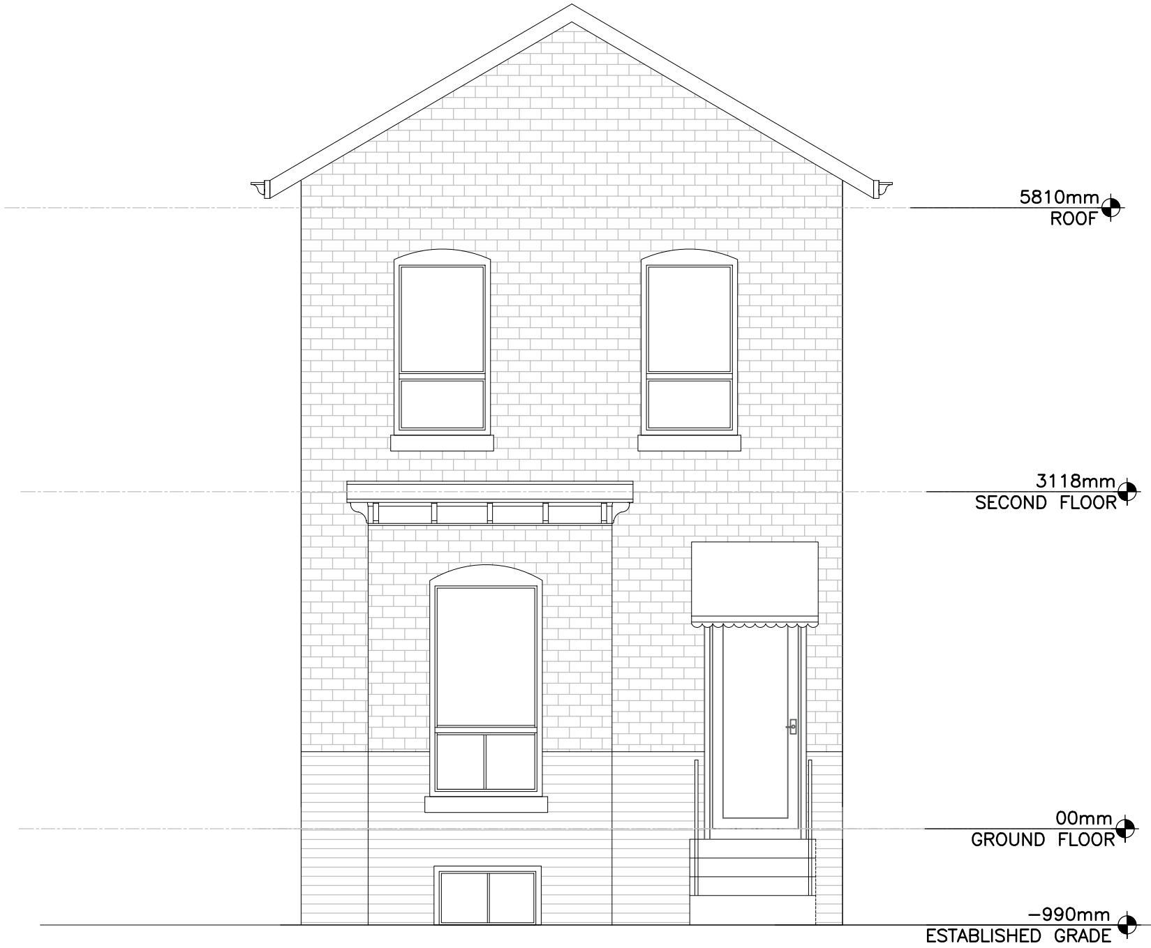
EXIST. NORTH ELEVATION 1 SCALE = 1:50 A2.01
