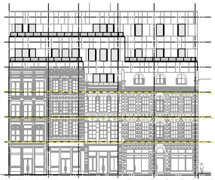
PROPOSED DEVELOPMENT – King Street East Elevation [DPAI] – yellow line indicates the continuous floor plates of the new building – the only area where the new floorplates are not consistent with existing window sill heights is on the 3<sup>rd</sup> floor of 28 King Street East (Glassco Building)
