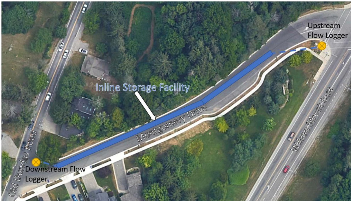
Figure 1.5: Locations of Sanitary Flow Loggers
