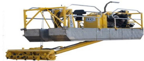
② SMALL-SCALE SEDIMENT REMOVAL SYSTEM DREDGE EQUIPMENT NOT TO SCALE
