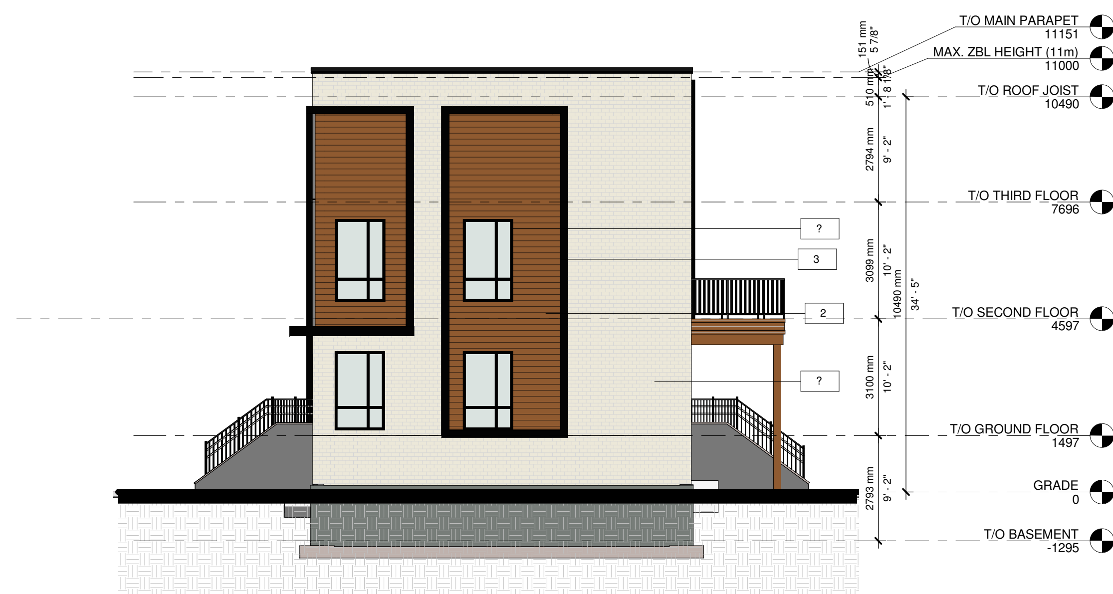
3 BLOCK 2 - EAST ELEVATION A202 1 : 100
