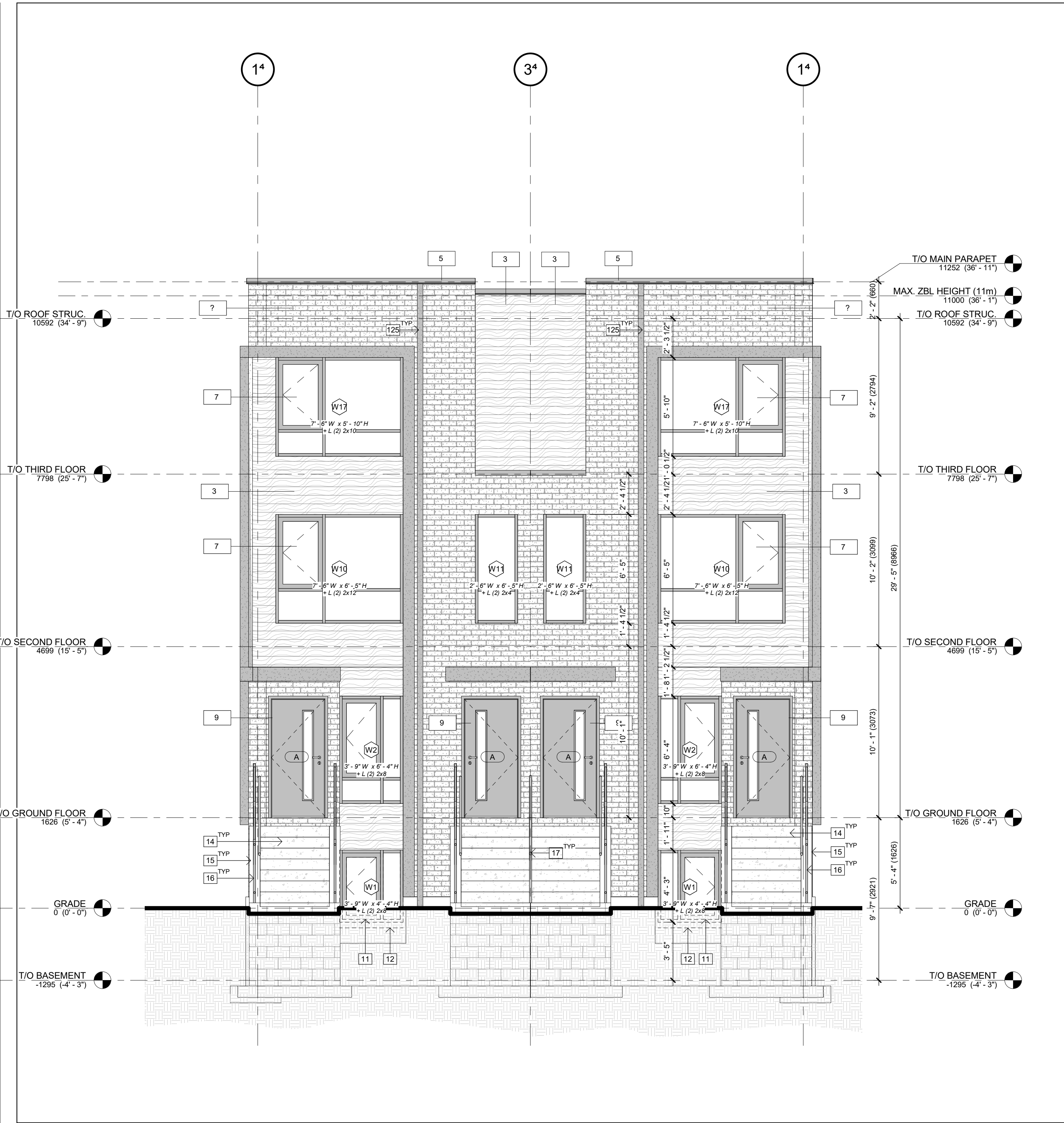
1 FRONT ELEVATION - SEMIS A200c 1/4" = 1'-0"
