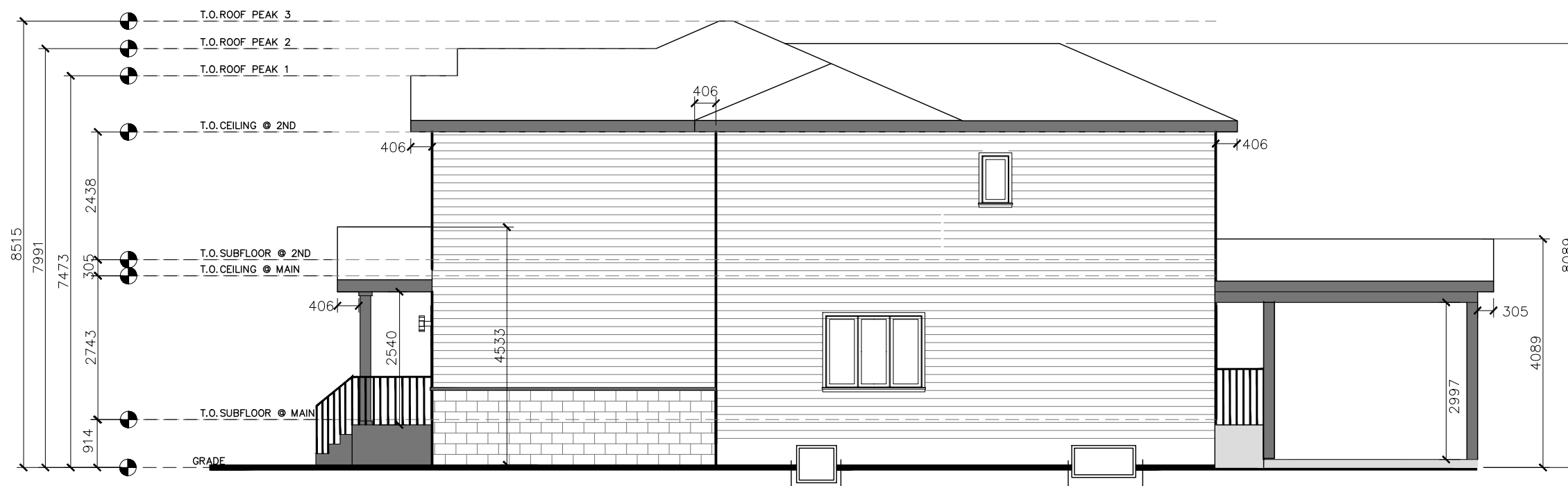
1 A2.01 FRONT ELEVATION Scale 1:100
