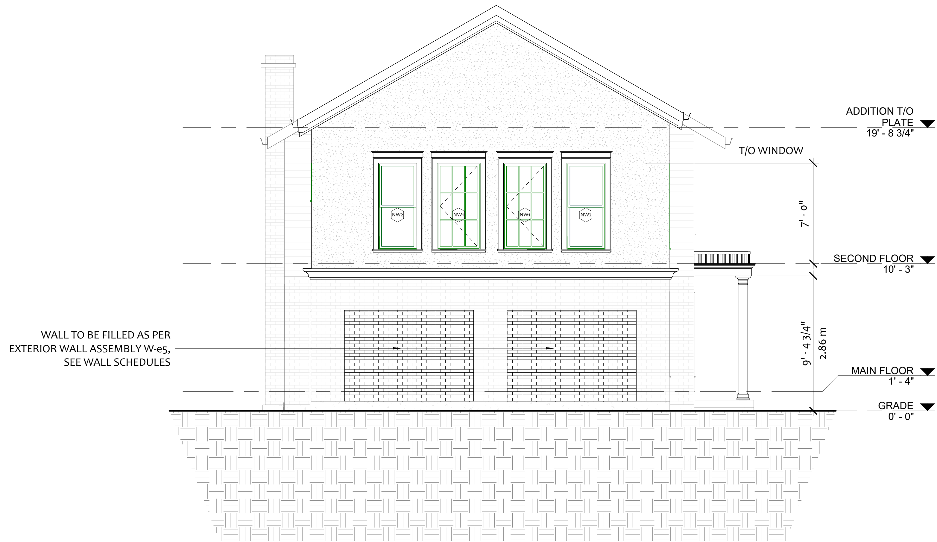
1 SOUTH ELEVATION A1.05 1/4" = 1'-0"
