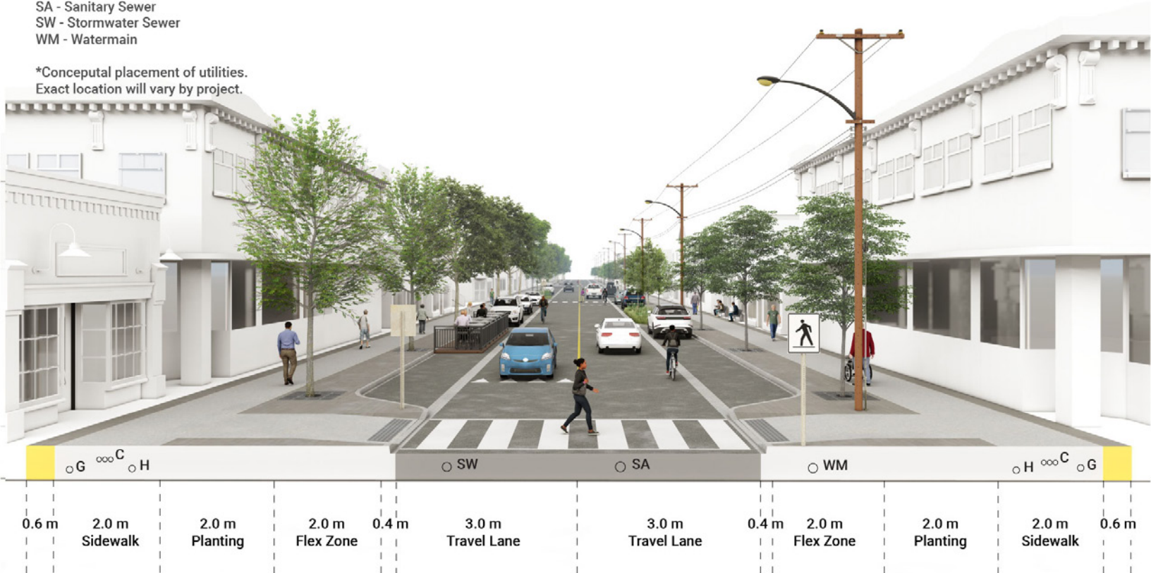
Typical Main Street Cross Section (20m ROW).
