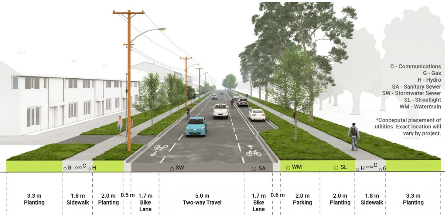
Typical Connector Cross Section (26m ROW)–Retrofit Scenario.
