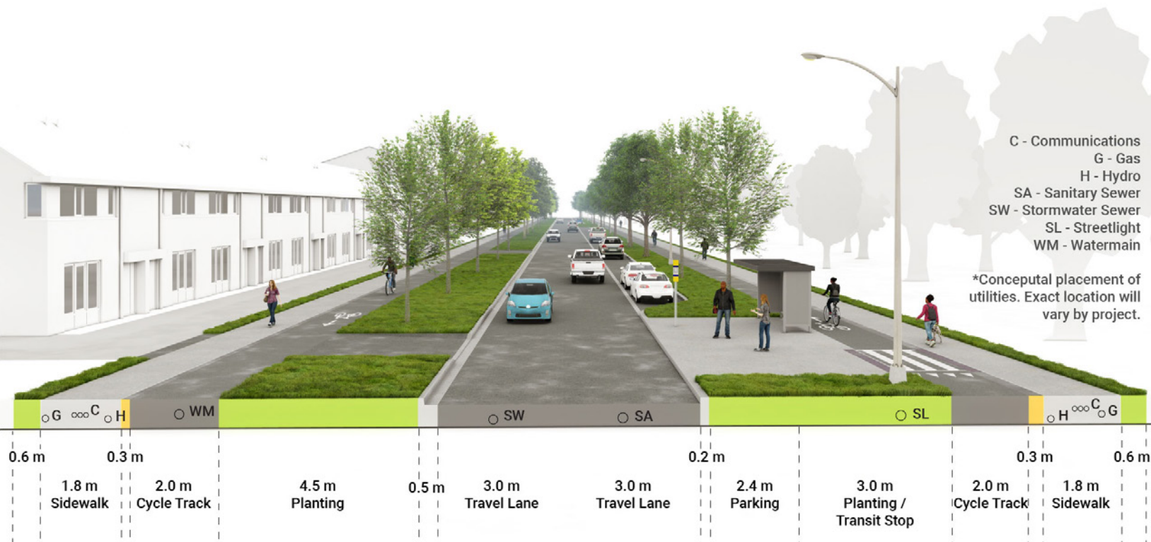
Typical Connector Cross Section (26m ROW) – New Construction.
