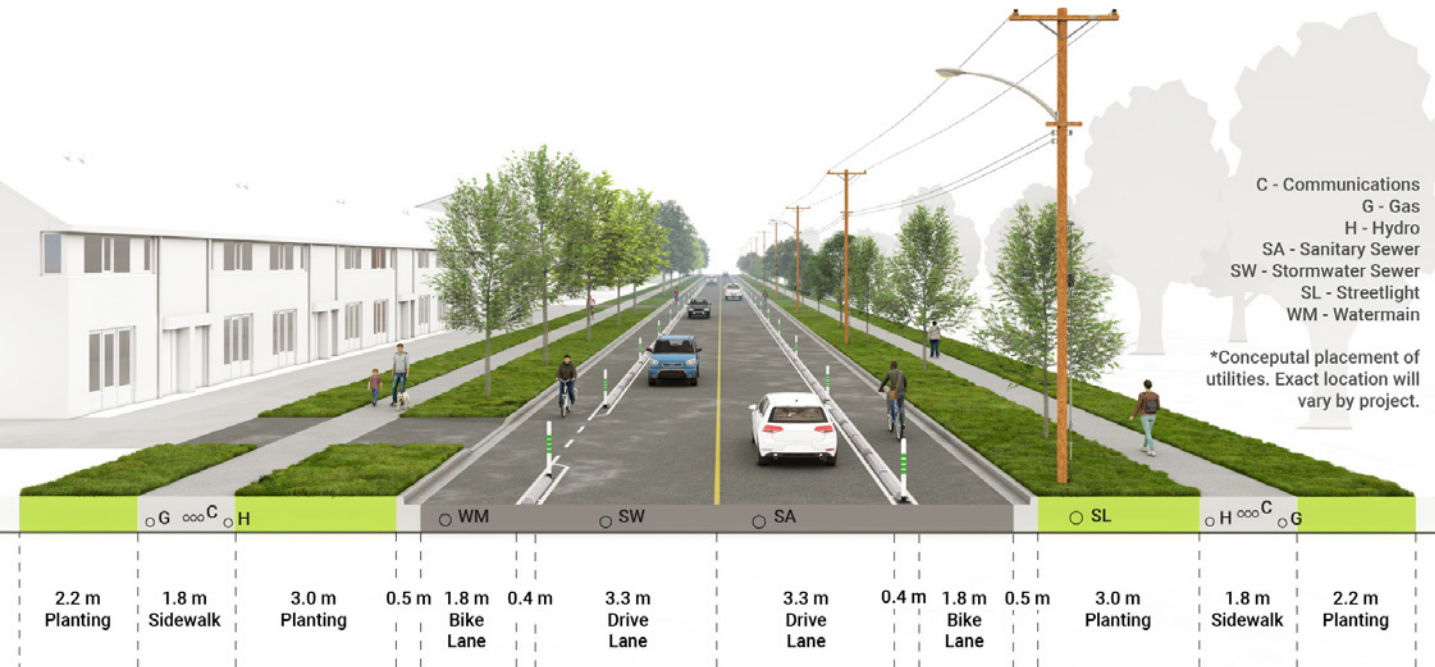
Typical Connector Cross Section (26m ROW)–Retrofit Scenario.
