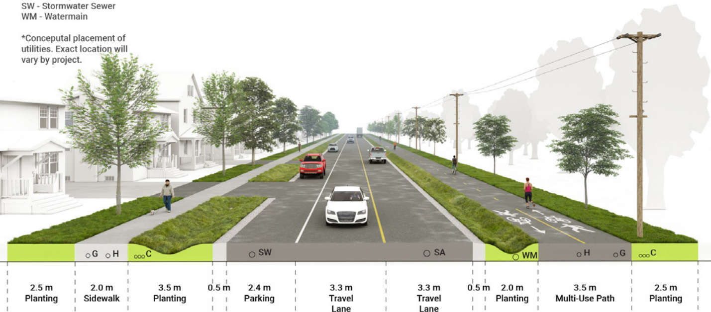
Typical Rural Settlement Area Cross Section with a Multi-Use Path (26m ROW)
