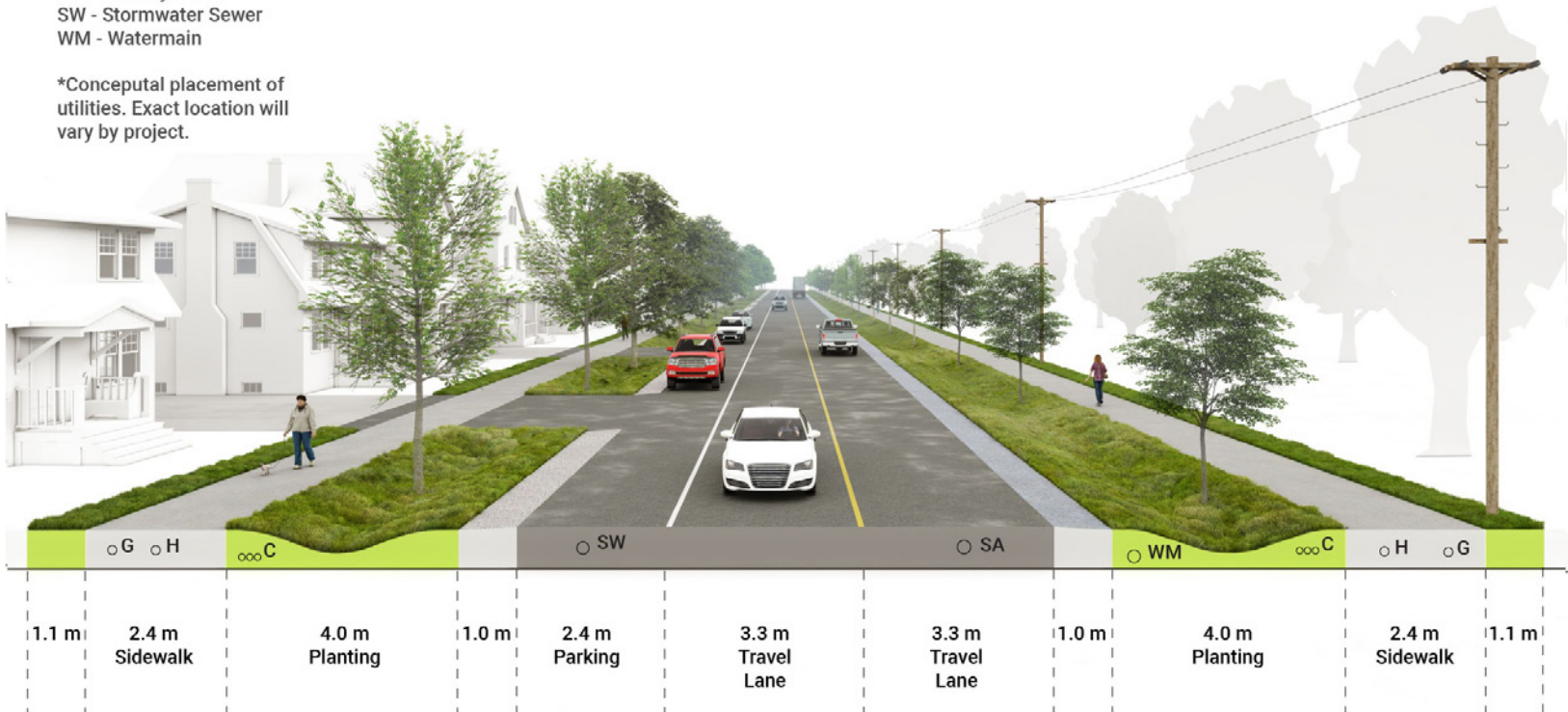
Typical Rural Settlement Area Cross Section (26m ROW)
