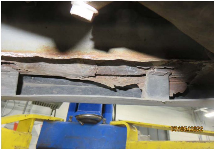
Figure 5. Vankleef #607 rusted hole in body panel. Image by FCC Inc.
