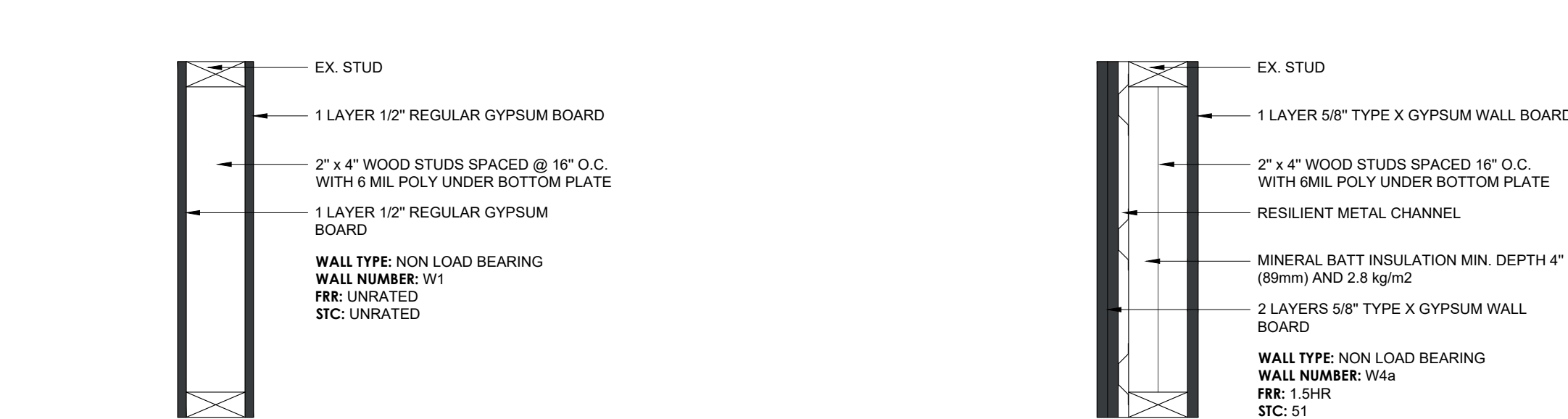
01 NEW: INTERIOR PARTITION WALL WITH GWB BOTH SIDES
