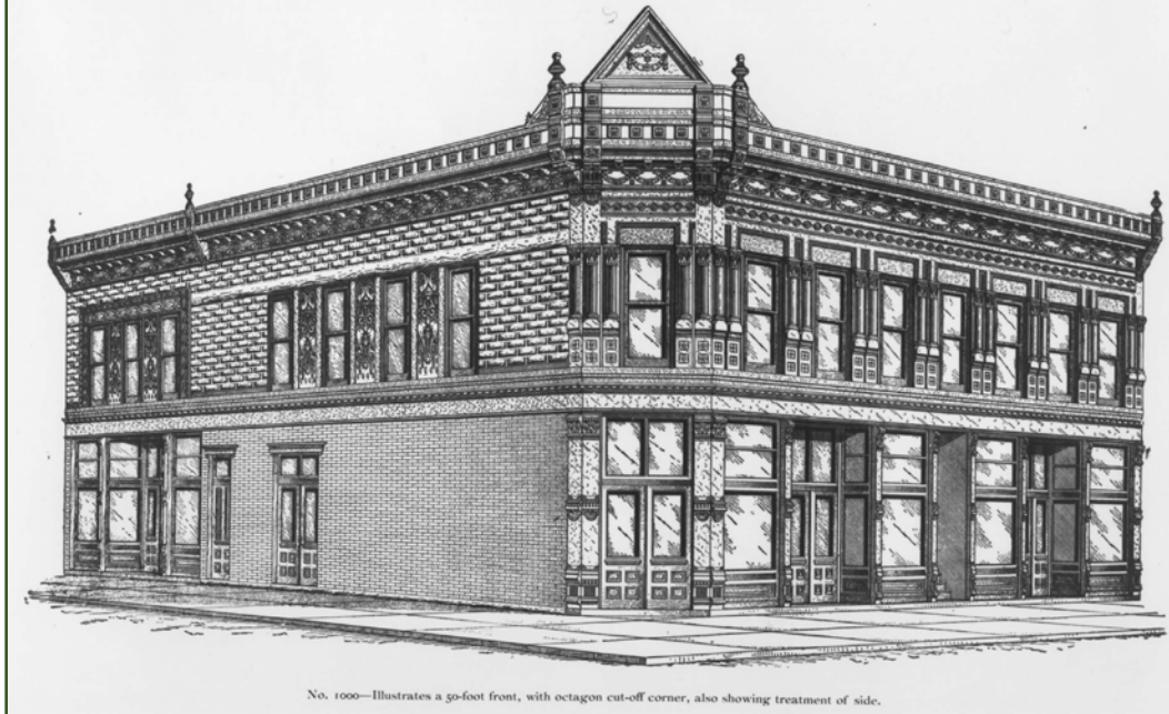
No. 1000—Illustrates a go-foot front, with octagon cut-off corner, also showing treatment of side.
