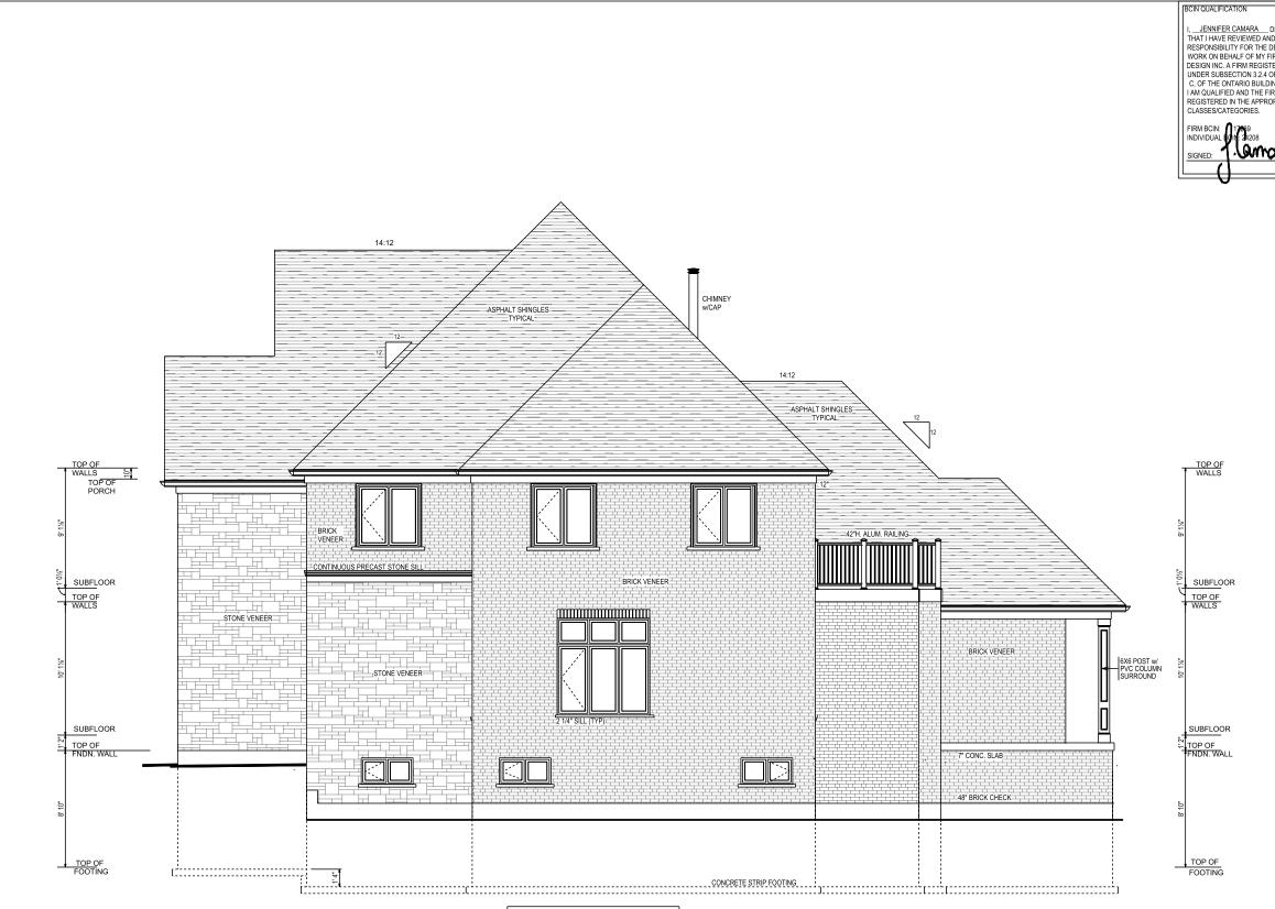
TOTAL EXPOSED BUILDING FACE: 1020 SQ.FT. ALLOWABLE UNPROTECTED OPENING AREA BASED ON 18'-7" SETBACK (32%): 326 SQ.FT.
