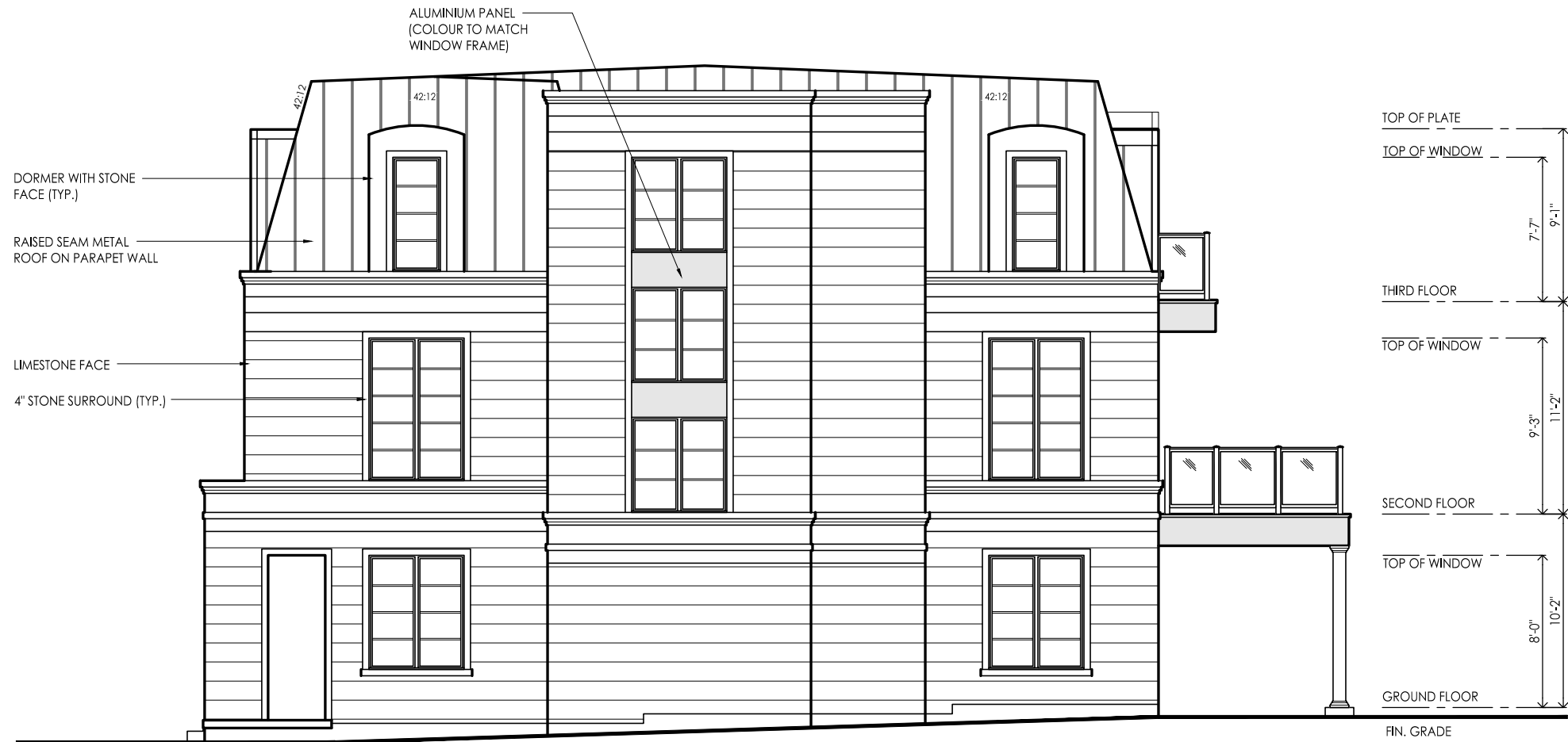
RIGHT SIDE ELEVATION 'A' CORNER
