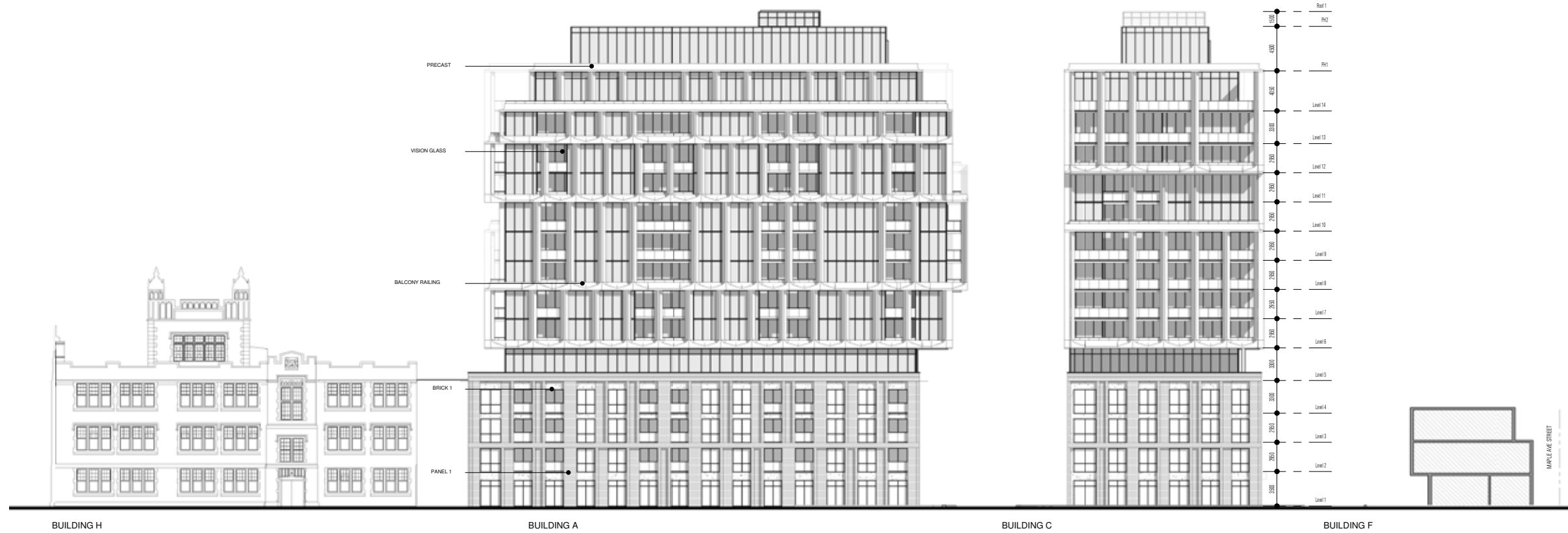
West elevation of Buildings H, A, and C (Graziani & Corazza Architects Inc., 2022).
