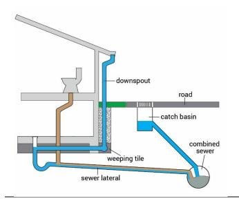
This illustrates typical drainage where a Combined Sewer is present, and a Joined Sanitary-Foundation Drain Lateral is in place.
