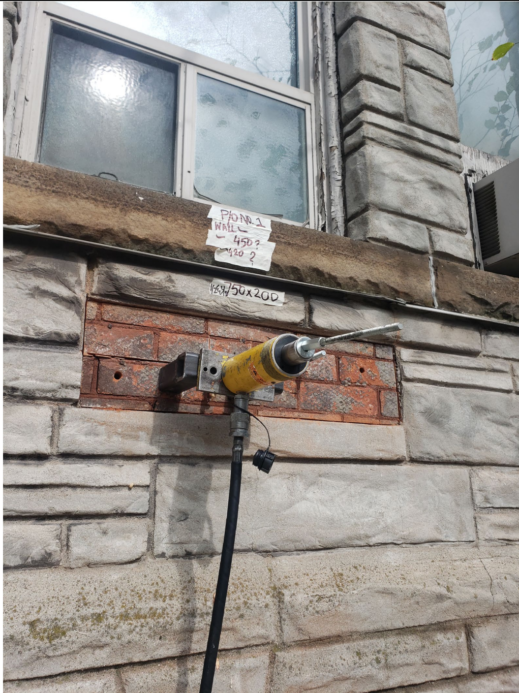
Photograph No. 37, showing a typical load test setup for Anchor Pull-Out Location No. 1.
