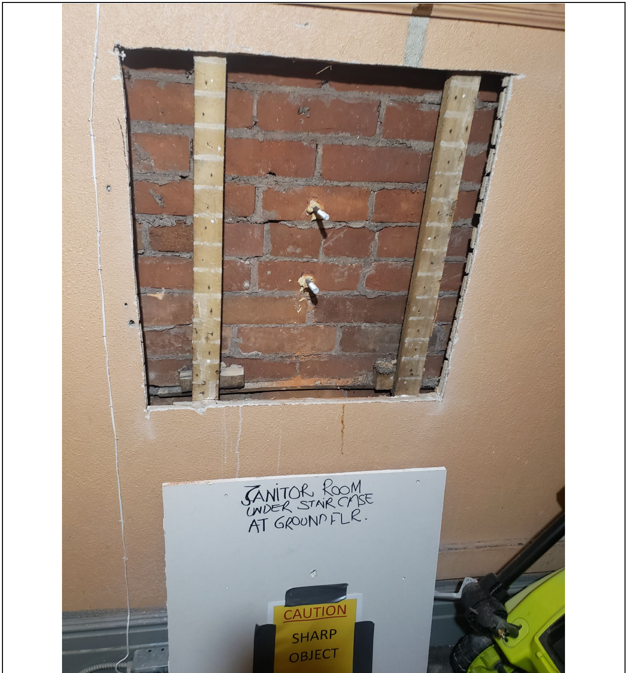
Photograph No. 41, showing anchor bolt installation for Anchor Pull-Out Location No. 4.
