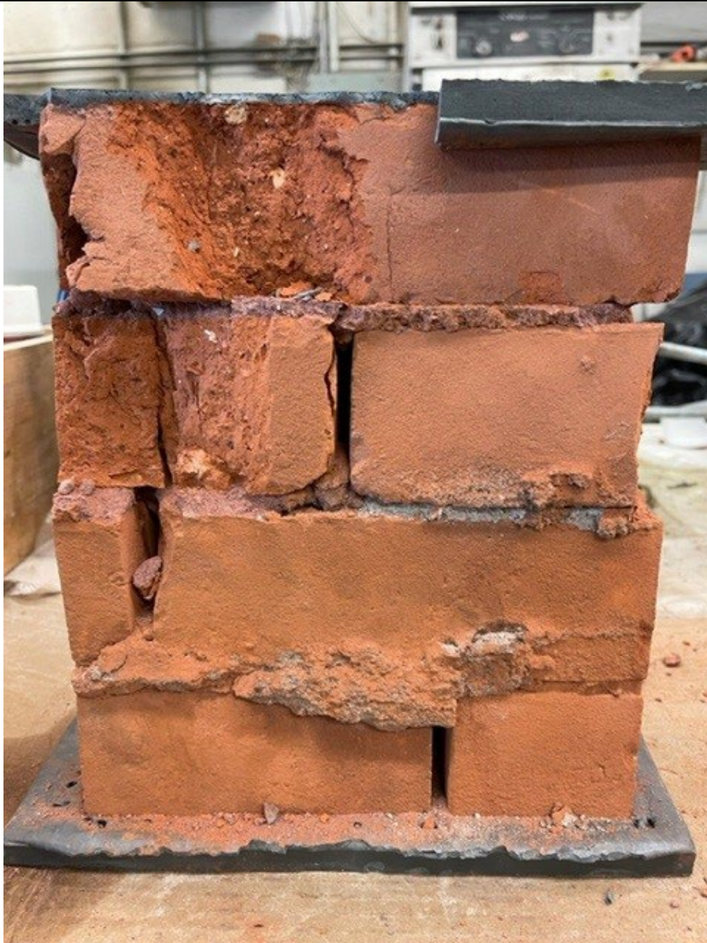
Photograph No. 15 Showing a view of Brick Prism No. 1 after testing.
