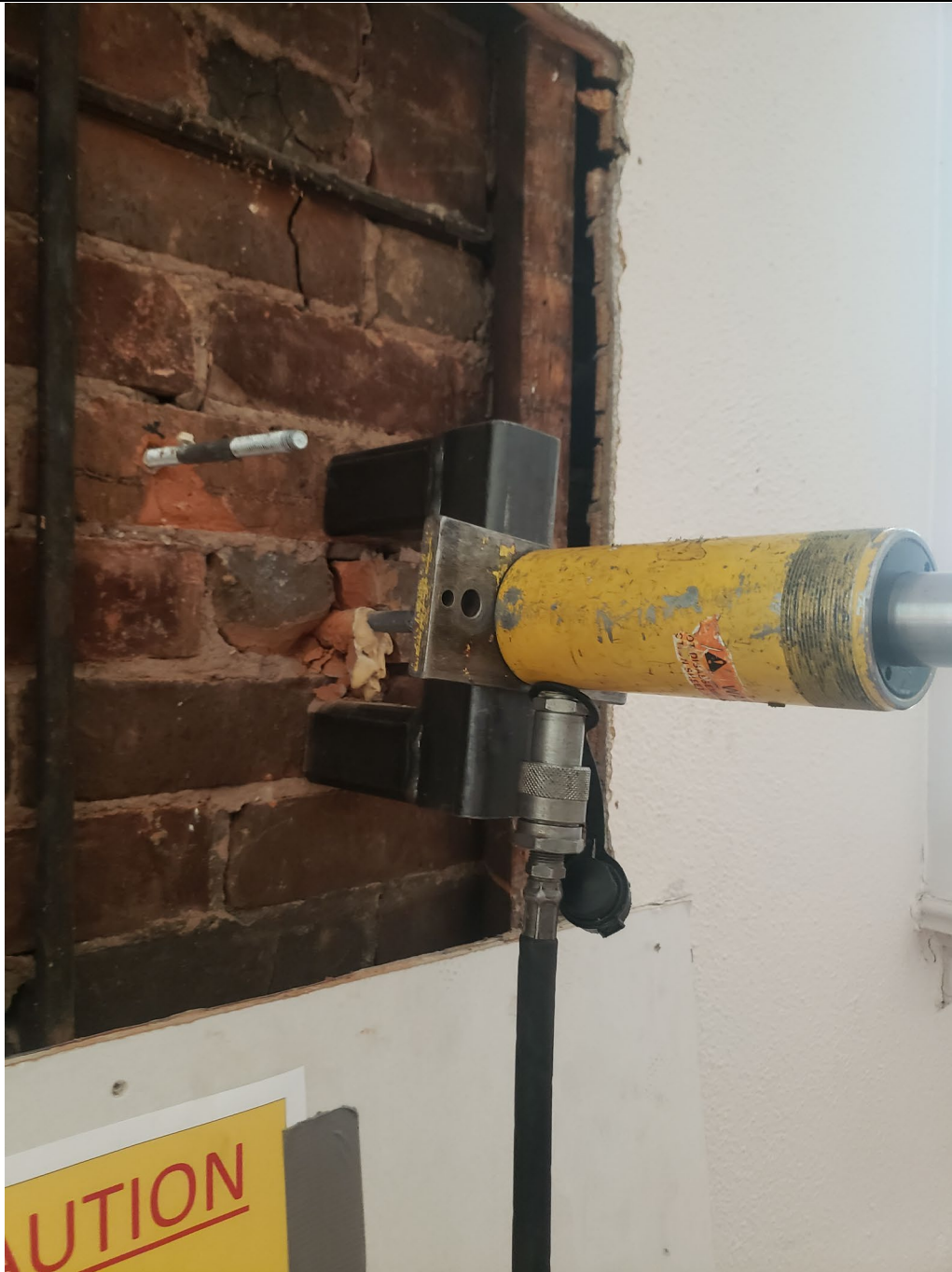
Photograph No. 43, showing pull-out failure of the brick for Anchor Pull-Out Location No. 5.
