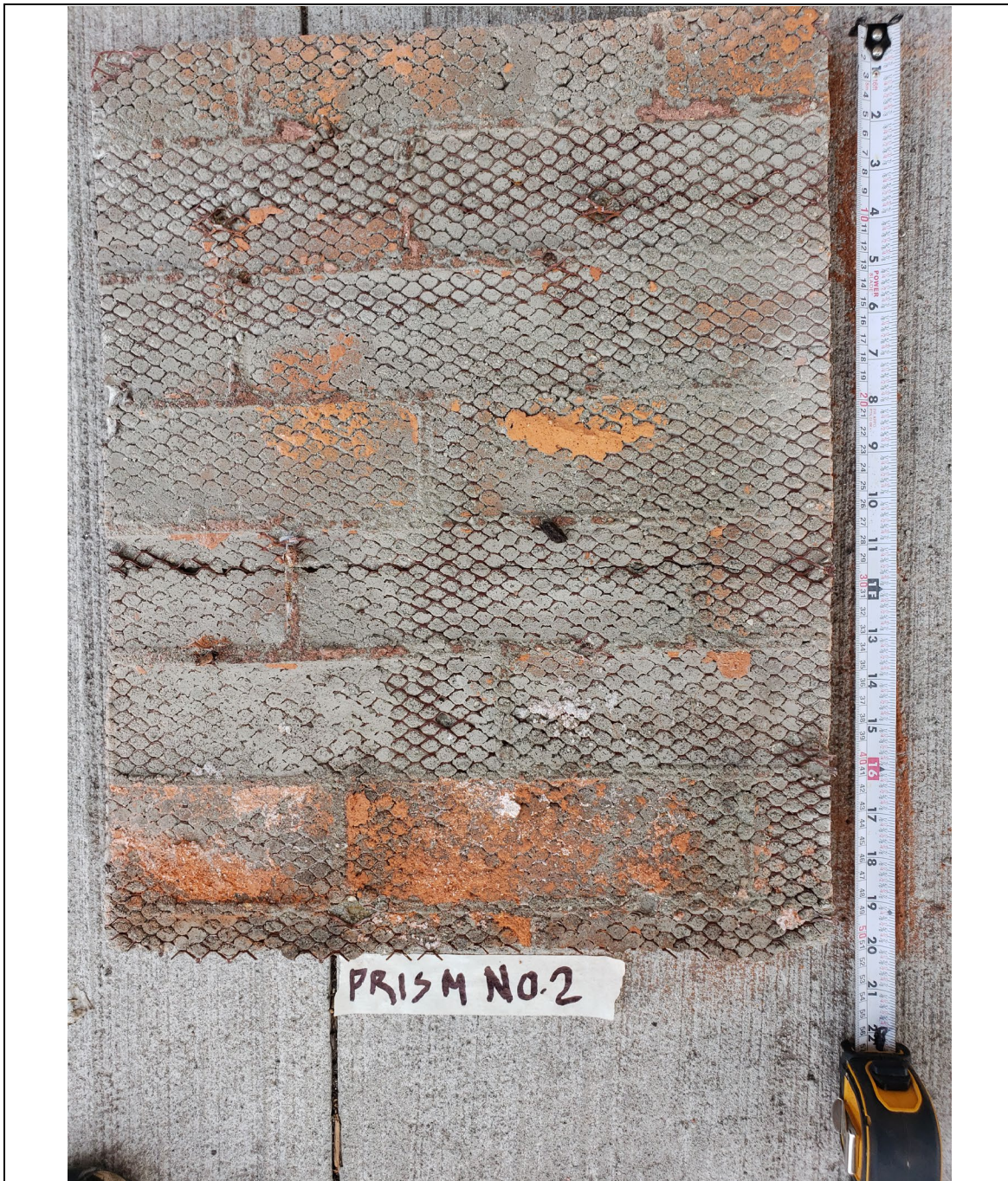
Photograph No. 7, showing the interior face of the stonework upon removal from the wall, for Brick Prism No. 2. Note the rusted expanded steel mesh, and adhering brick facing.
