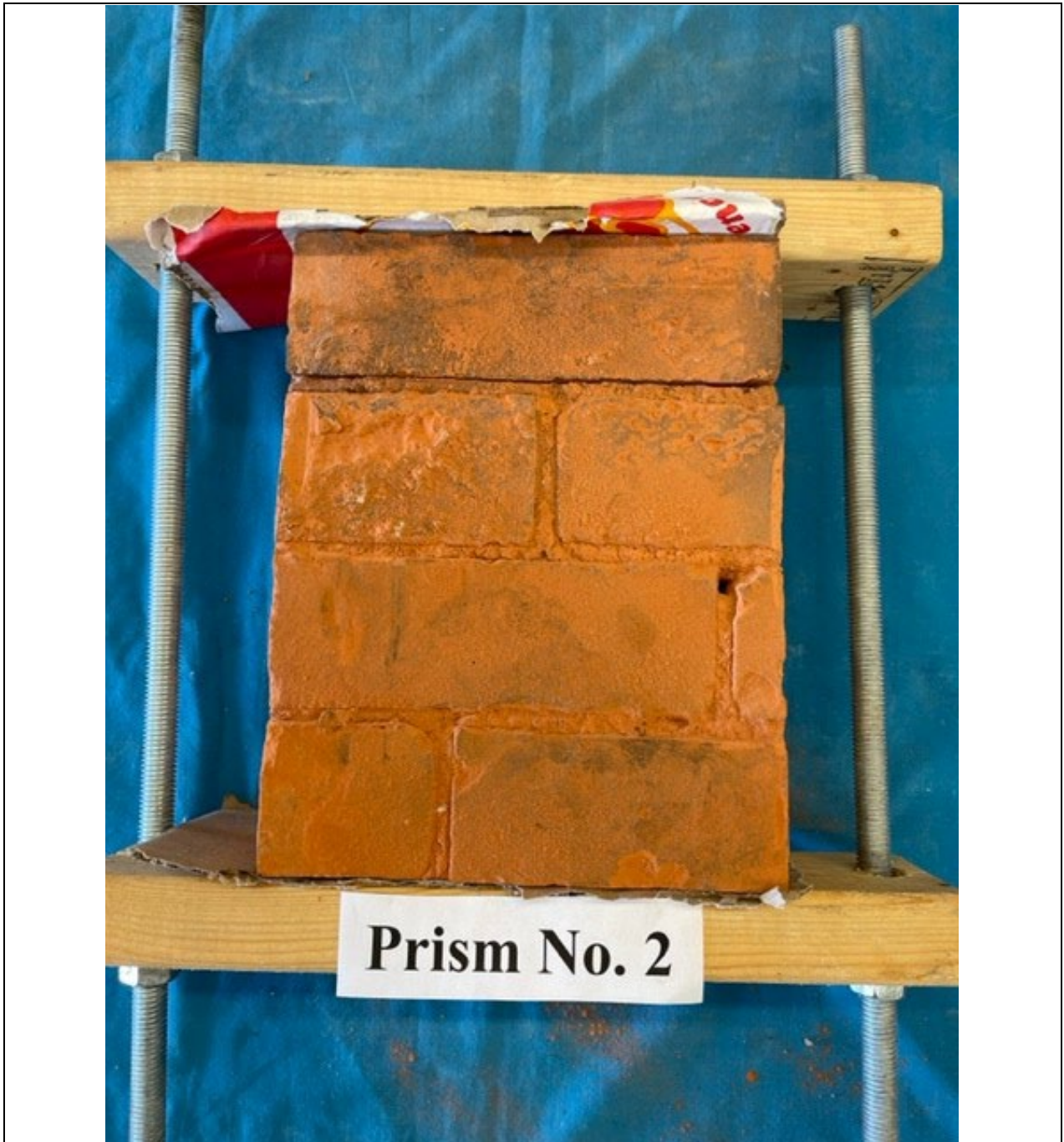
Photograph No. 13 Showing a view of Brick Prism No. 2 in the wood clamps to keep the sample in an intact condition
