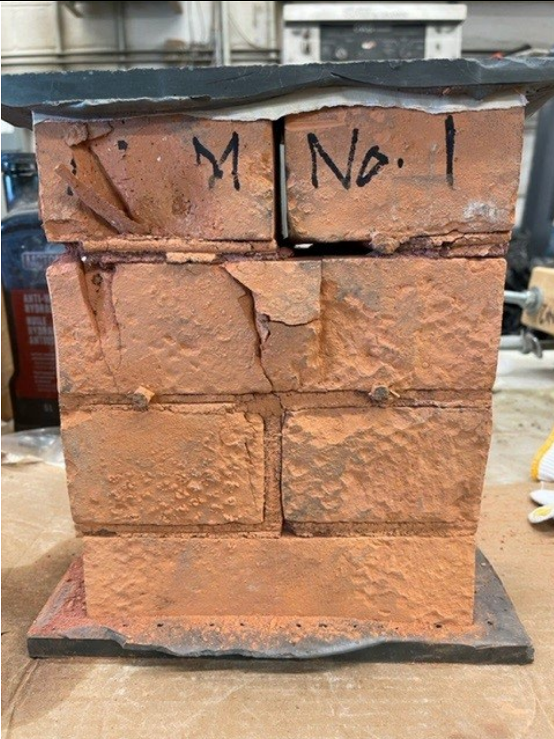
Photograph No. 12 Showing a view of Brick Prism No. 1 after testing.
