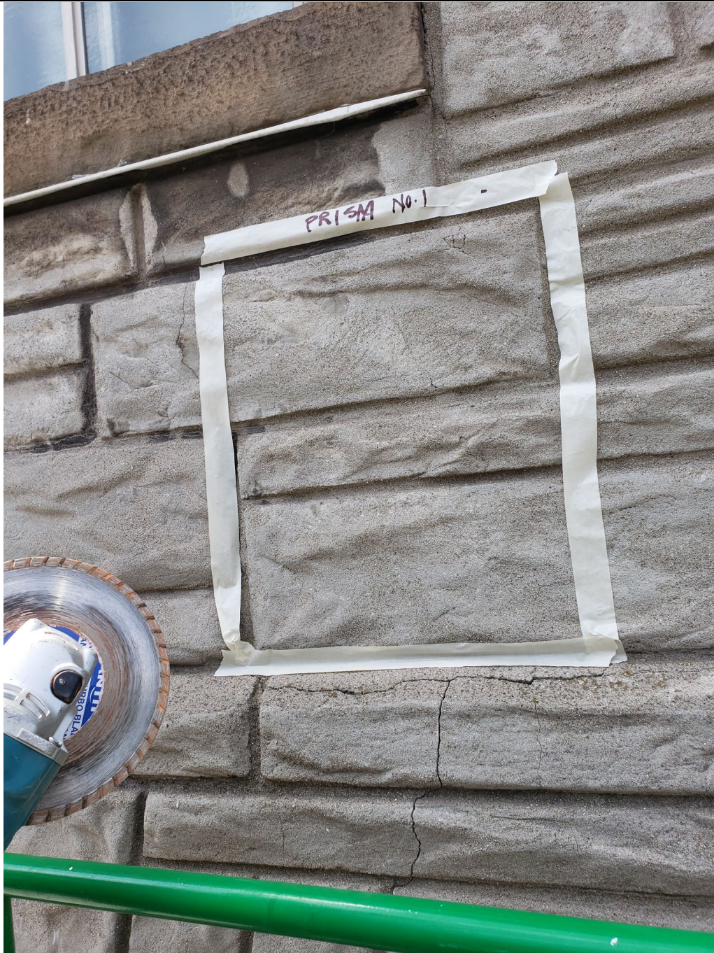
Photograph No. 3, showing test location for Brick Prism No. 1. Note the horizontal and vertical cracking seen in the stone work.
