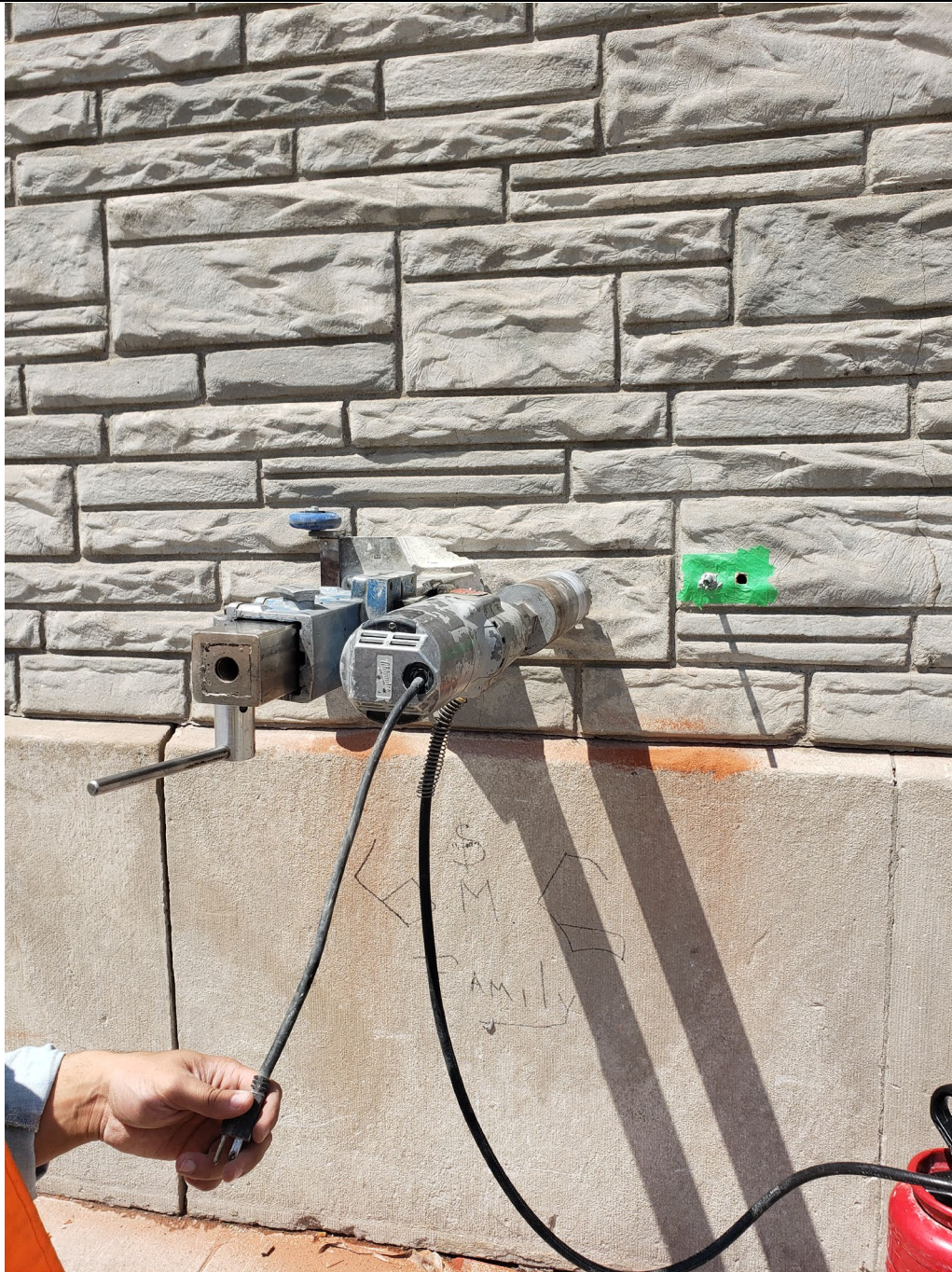
Photograph No. 45, showing a view of a typical drilling machine setup (Core No. 2).
