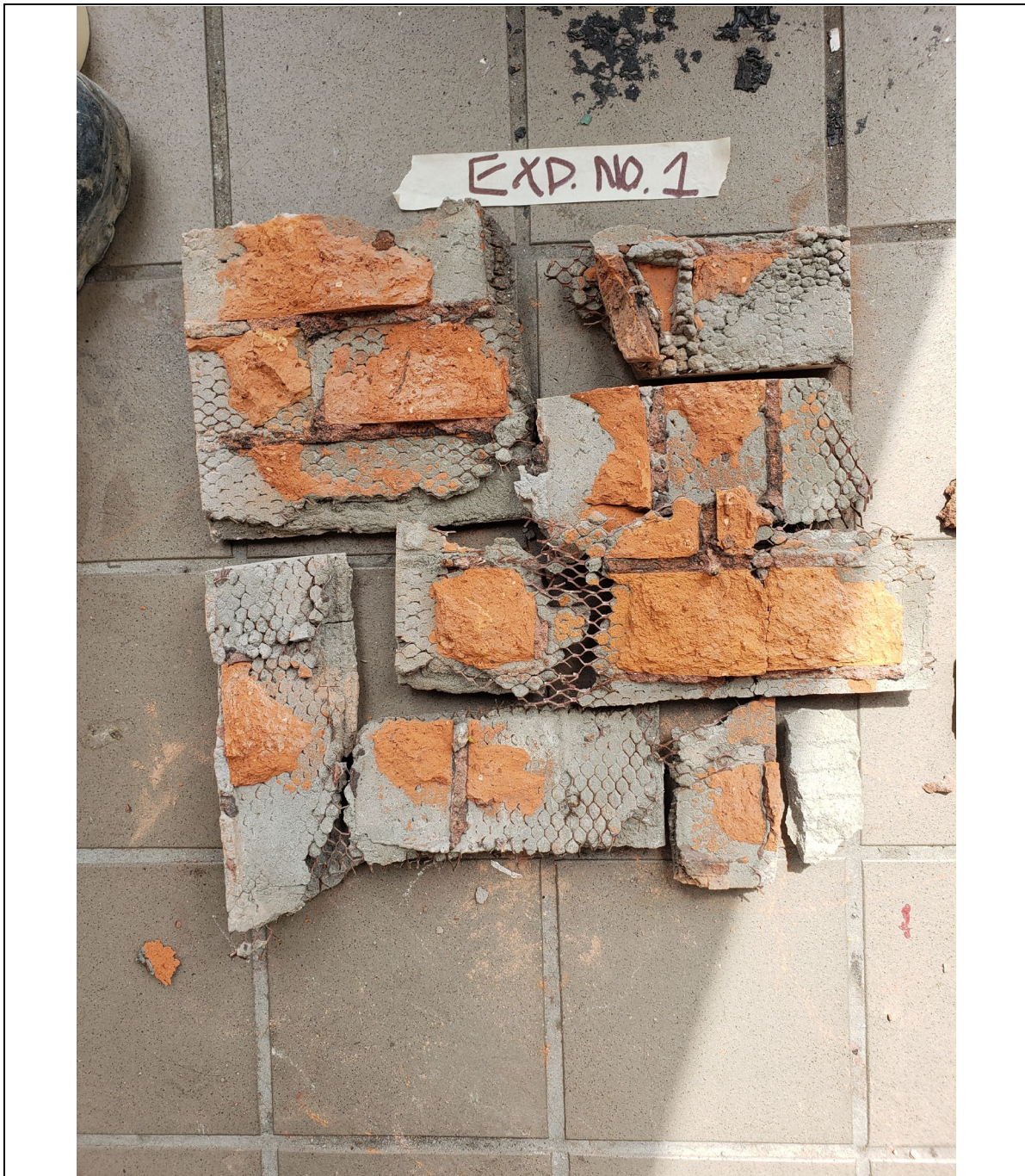
Photograph No. 18, showing the interior view of the removed stonework for Exploratory Opening No. 1. Note the spalled brick, and rusted expanded steel mesh.
