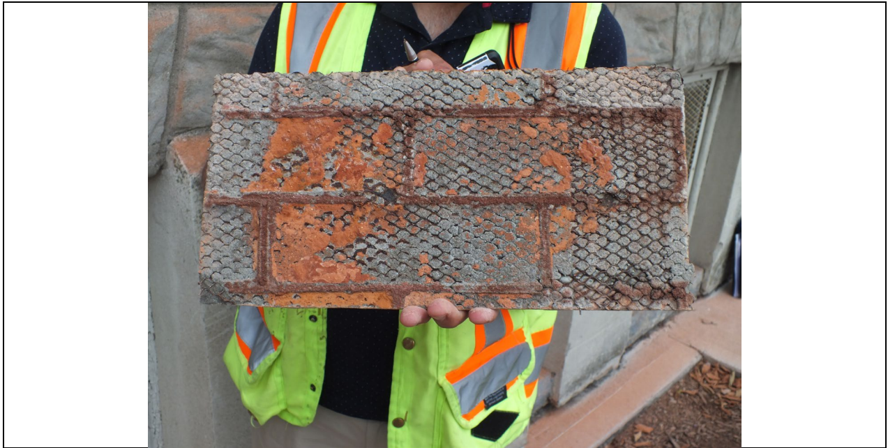
Photograph No. 38, showing the back side of the 1 st . piece stonework for Anchor Pull-Out Location No. 1. Note the rusted expanded steel mesh and rusted concrete steel nails, and spalled brick pieces.
