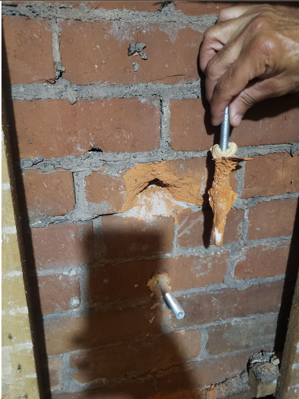
Photograph No. 42, showing conical failure of the brick for Anchor Pull-Out Location No. 4.
