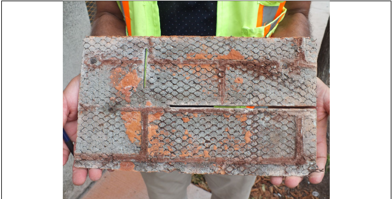
Photograph No. 39, showing the back side of the 2 nd . piece stonework for Anchor Pull-Out Location No. 1. Note the rusted expanded steel mesh and rusted concrete steel nails, and spalled brick pieces.
