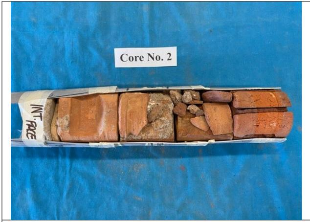
Photograph No. 49, showing an interior view of Core No. 2. Note the wall thickness is made up of four (4) wythes of brick.
