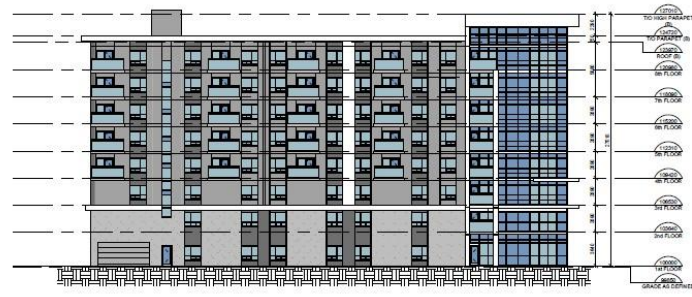
2 EAST ELEVATION - BUILDING B A403 1:200
