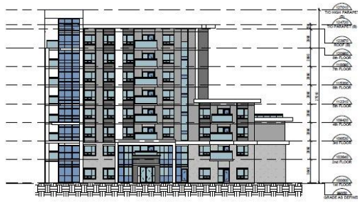
4 NORTH ELEVATION - BUILDING B A403 1:200
