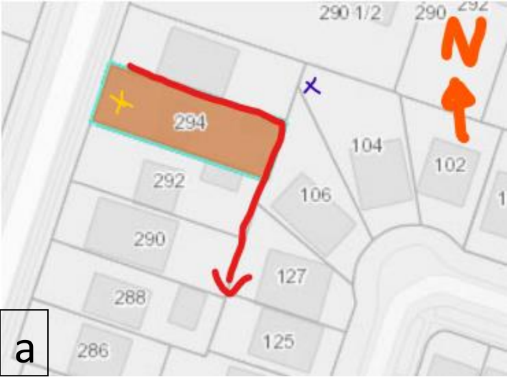
Fig. 4. (a) Location of retaining wall (red line) and catch basins (blue and yellow X). (b) Downward slope of 294 Green Road with the catch basin (yellow) near the high point compared to even grade of 296 Green Road.
