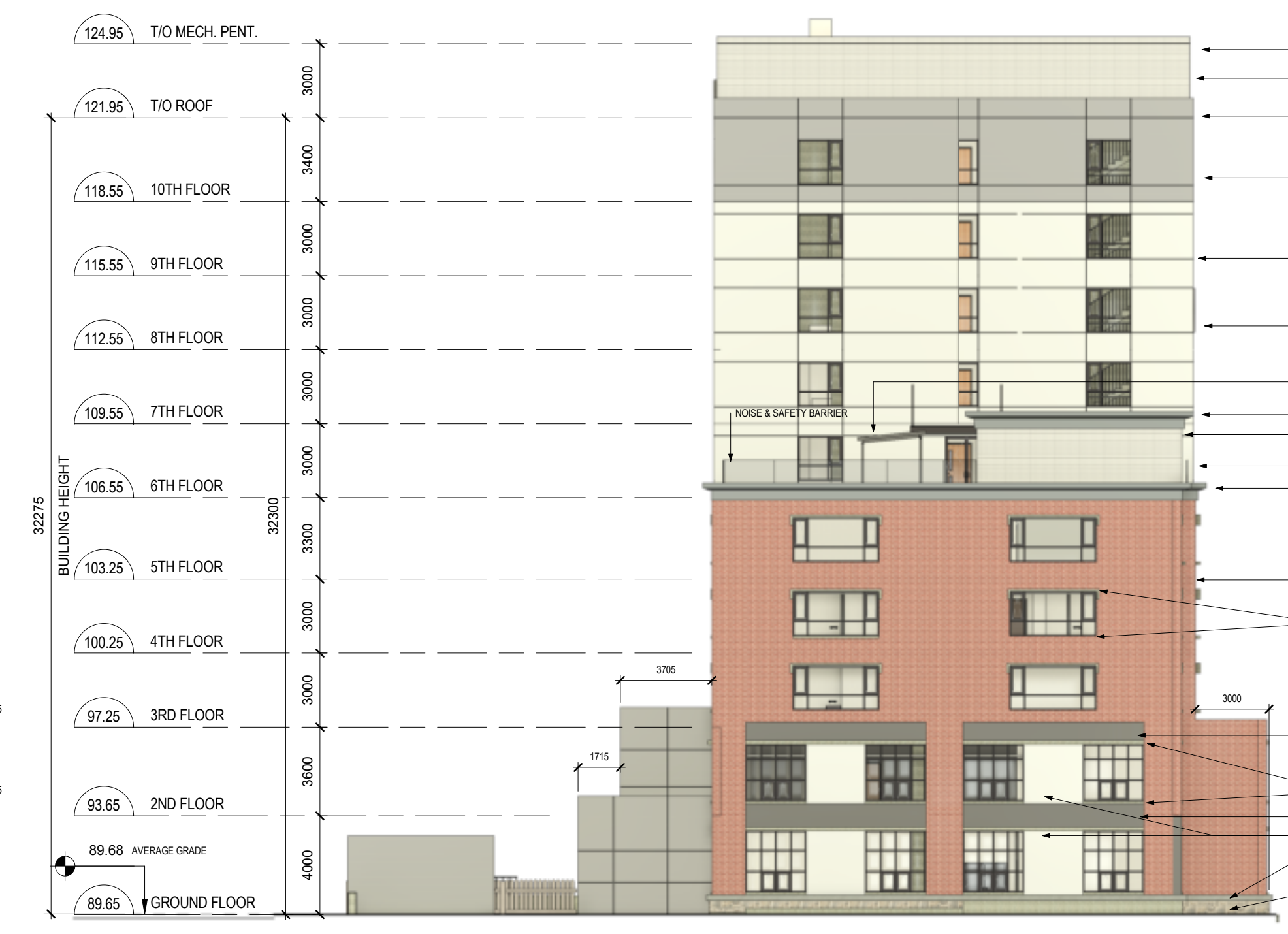
4 SOUTH ELEVATION - SPA A-3.1 1 : 200
