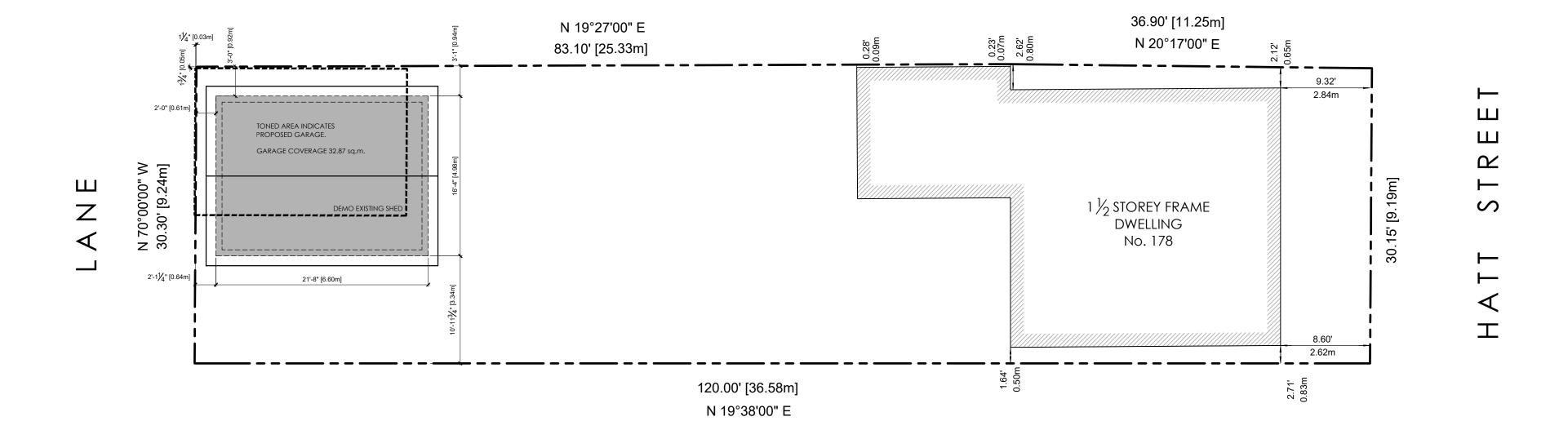
LOT AREA: 339.01 m<sup>2</sup> (3,649.03 ft<sup>2</sup>) HOUSE FOOTPRINT: 86.88 m<sup>2</sup> (935.16 ft<sup>2</sup>) PROPOSED GARAGE: 32.87 m<sup>2</sup> (353.81 ft<sup>2</sup>) THIS DRAWING IS NOT TO BE SCALED.
