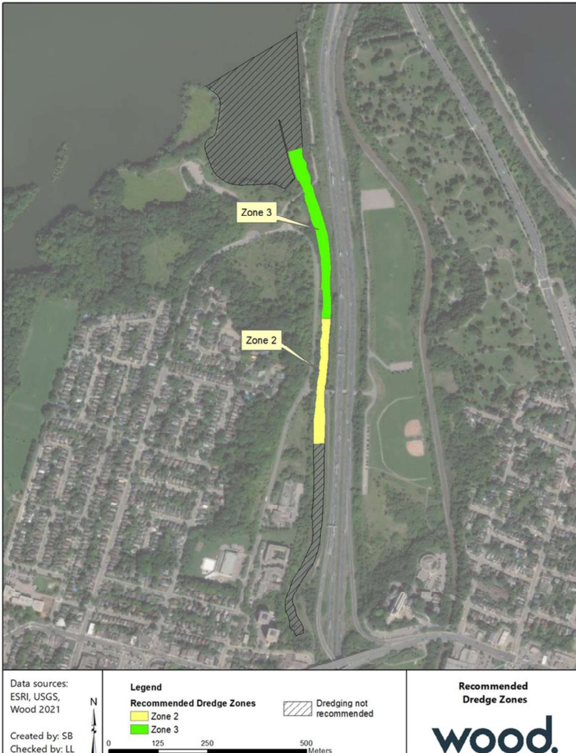
Figure 2.3: Recommended Dredge Zones 2 and 3.
