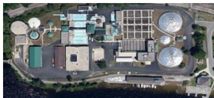
Traverse City WWTP, USA ADF 27 MLD (7.1 MGD) MDF 64 MLD (17 MGD) Commissioned 2005 Proven membrane life 16 years
