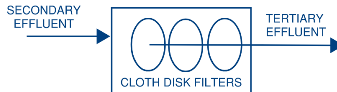
Figure 4-11: Typical Cloth Disk Filter Process Schematic with an Outside-In Flow Pattern
