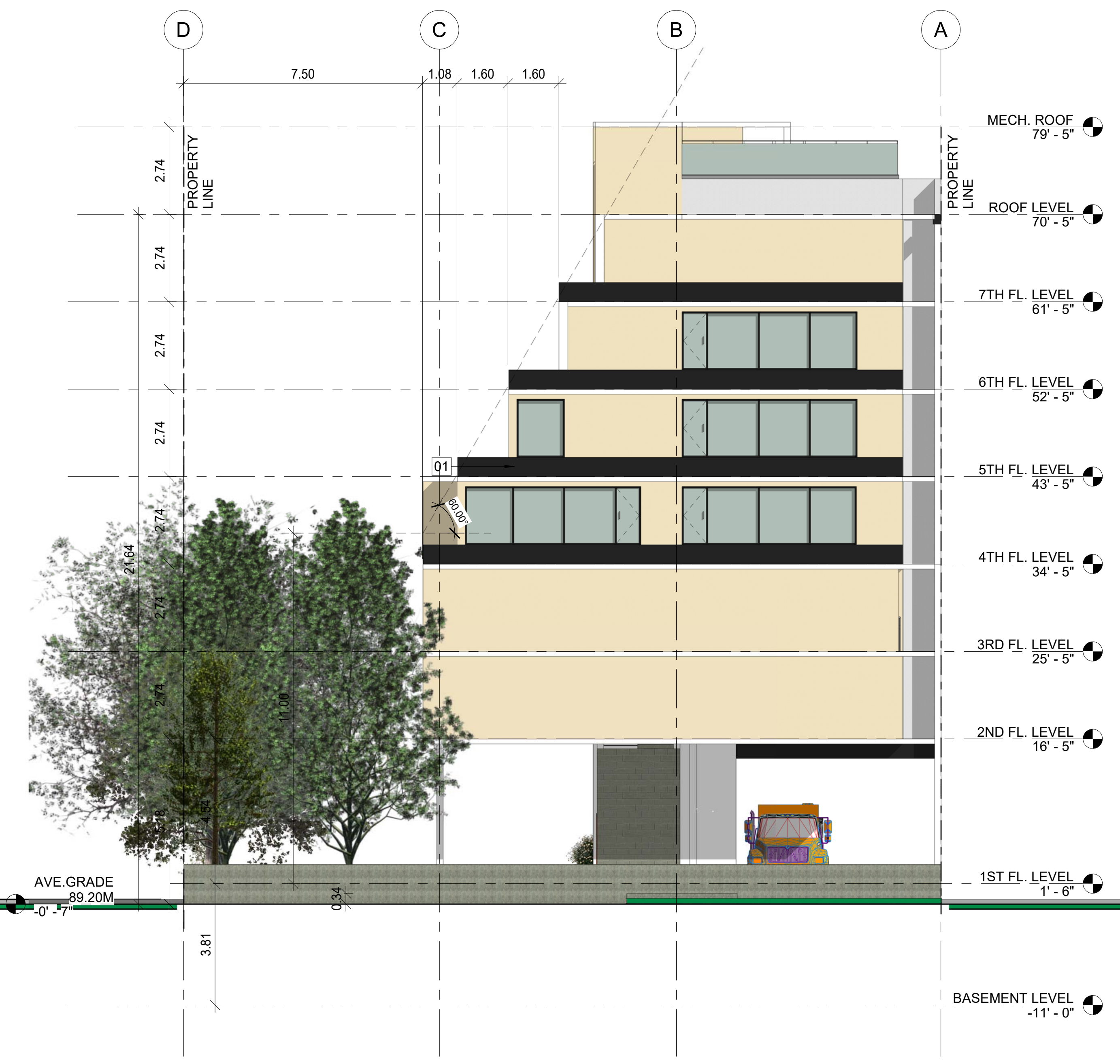
2 NORTH REAR ELEVATION A3.0 1/8" = 1'-0"
