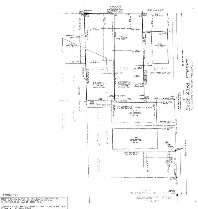
COORDINATES CAN NOT, IN THEMSELVES, BE USED TO RE-ESTABLISH CORNERS OR BOUNDARIES SHOWN ON THIS PLAN. DISTANCES ON THIS PLAN ARE GROUND AND CAN BE CONVERTED TO GRID BY MULTIPLYING BY THE COMBINED SCALE FACTOR OF 0.99968203
