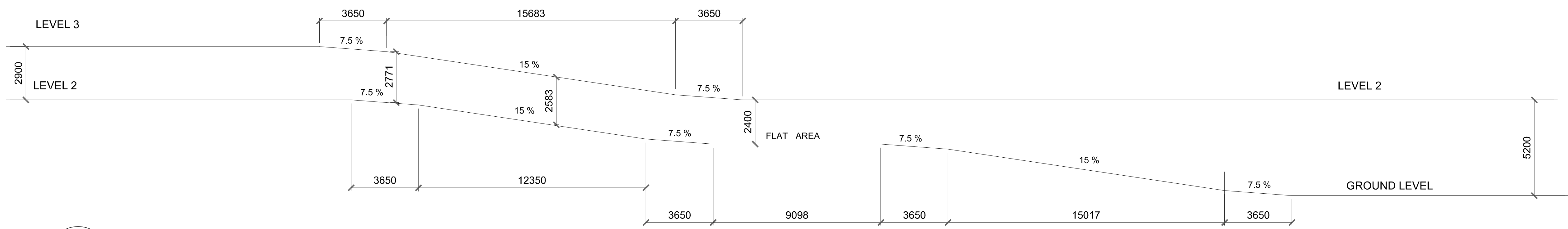
2 RAMP FROM GROUND TO SECOND SECTION A104
