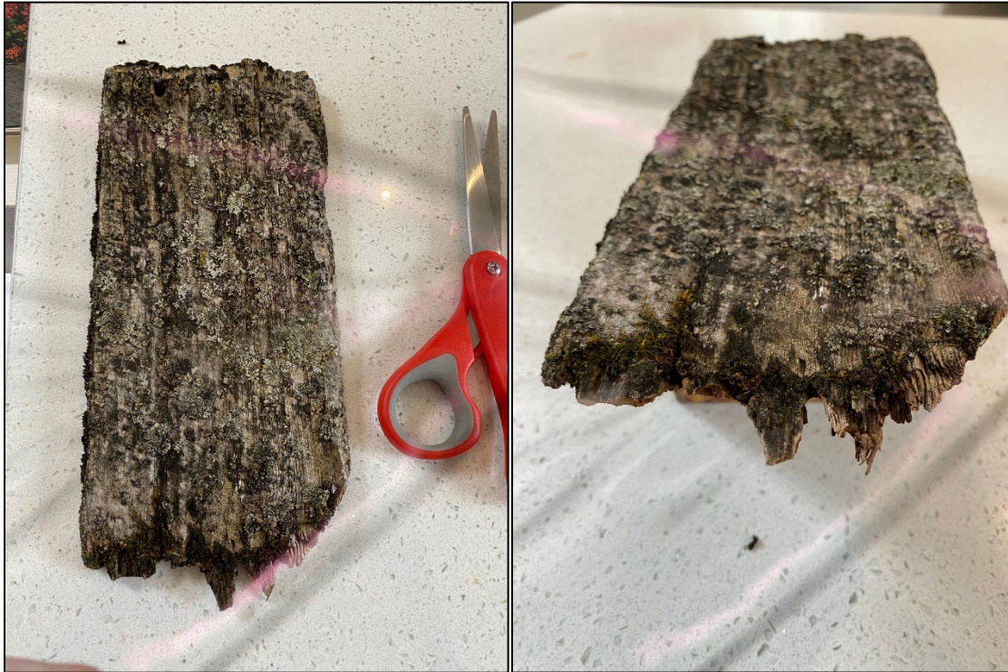
Figure 6: Existing roof shingle that blew off of home during high winds – shows level of deterioration.
