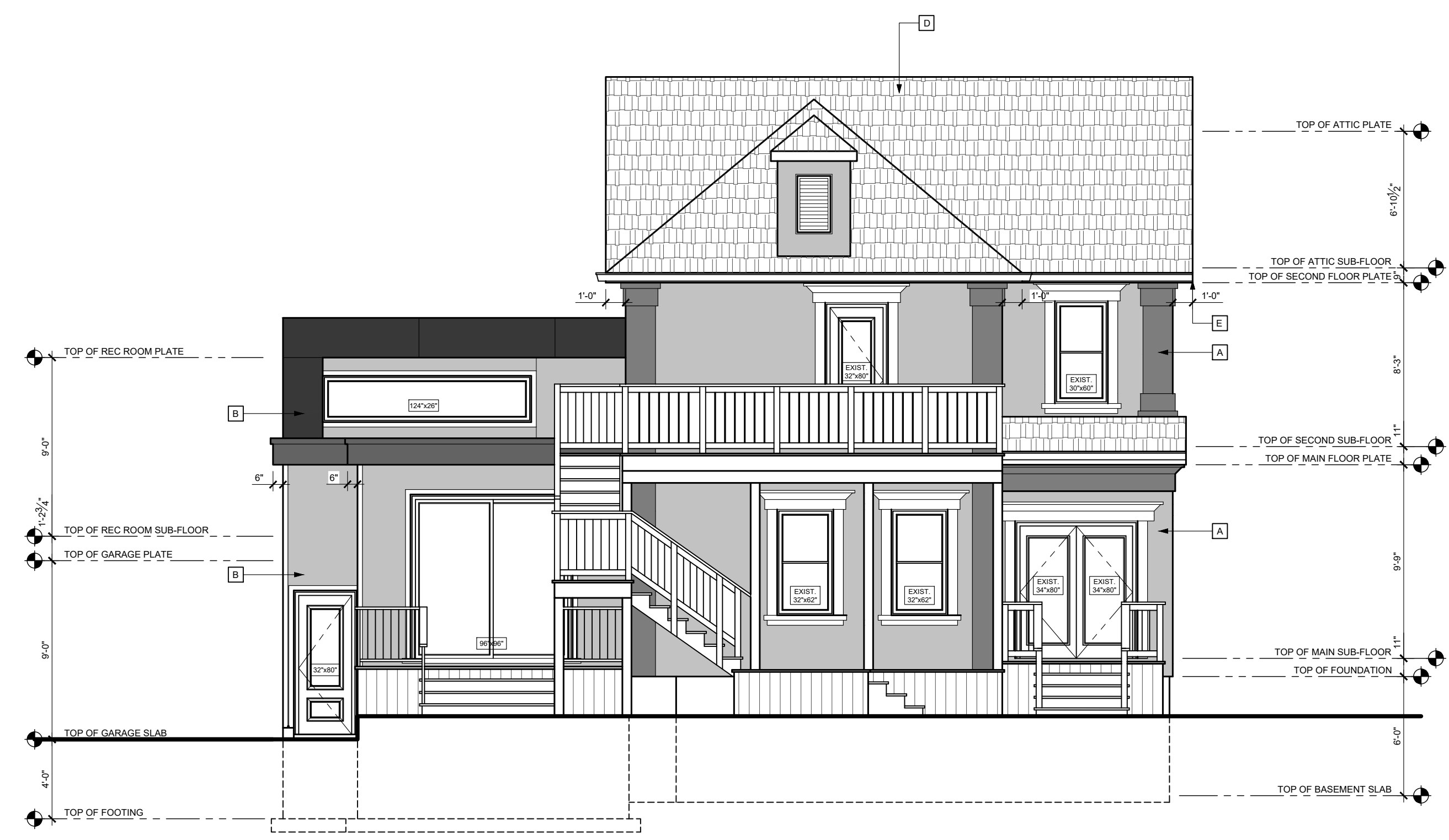
REAR ELEVATION SCALE 3/16" = 1' - 0"
