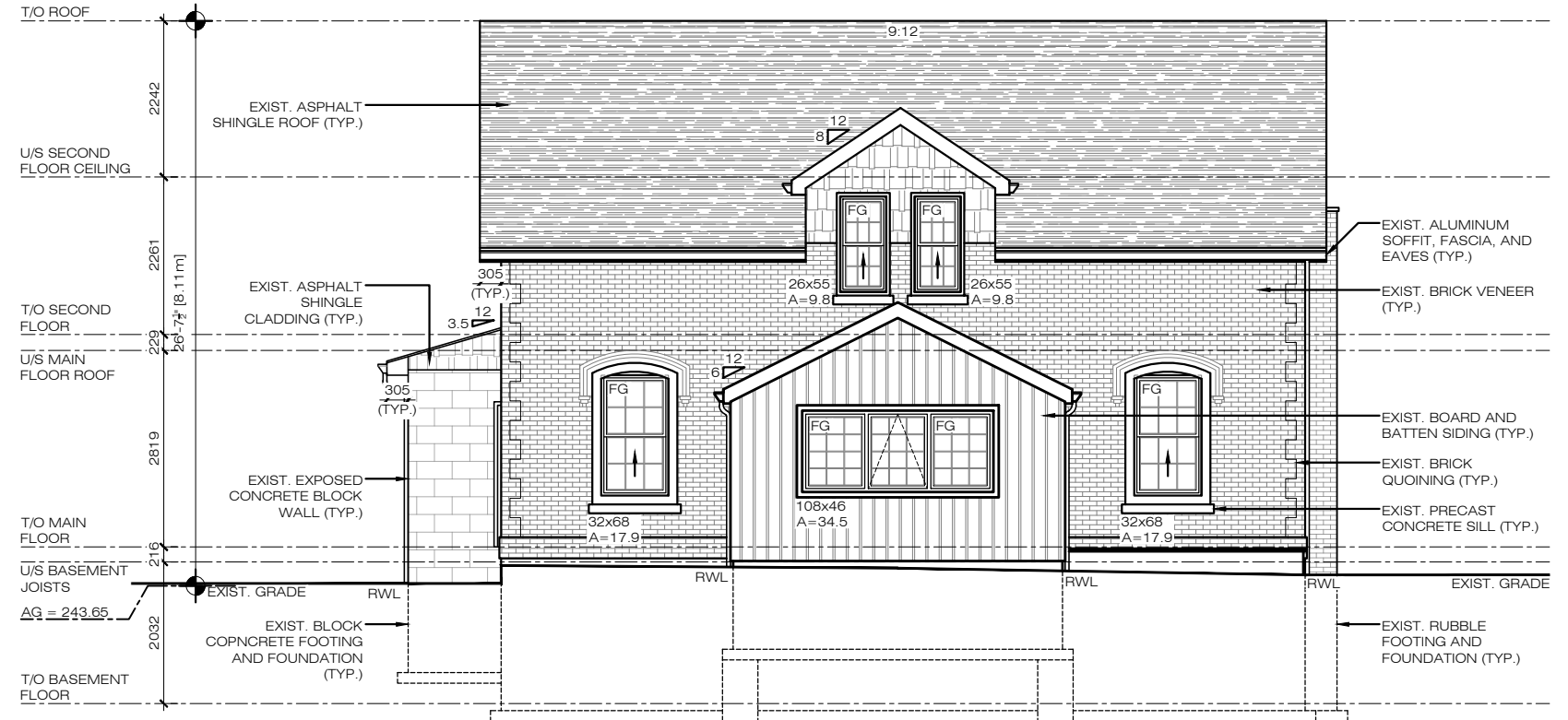
EXISTING LEFT SIDE ELEVATION
