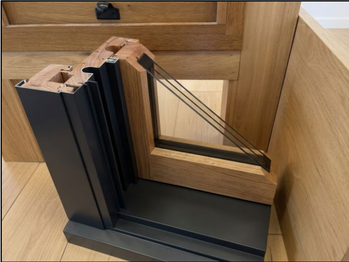
Figure 3: Cross-section of proposed windows, wood sill construction with wood interior and aluminum clad exterior frame (Proponent, 2026)
