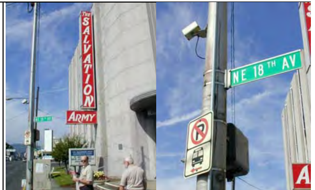
Microwave sensors are aimed at the crosswalks to track pedestrians. Source: Designing for Pedestrian Safety.
