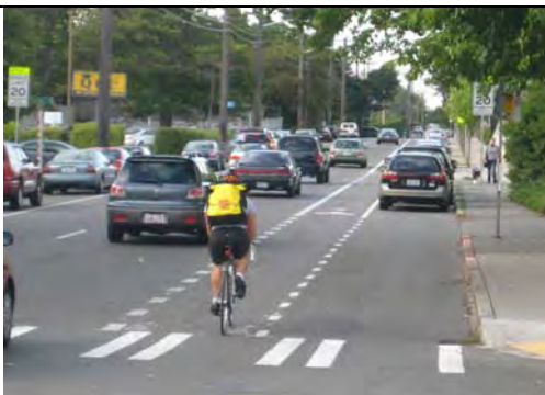
Bicycle lane and parked cars can provide a buffer between sidewalk and vehicle lanes.
