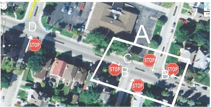
The existing area has a 4 way stop at a badly skewed intersection (A), no brake lines (B), no wheel chair ramp (C) at "stop" area and little traffic flow control on a busy street (D).
