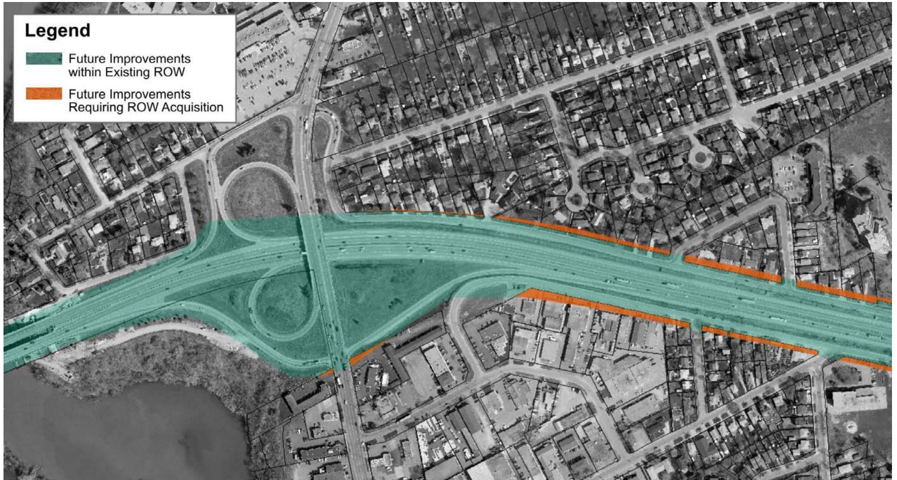
Exhibit 4-31: Sample Application of Interchange Widening Template
