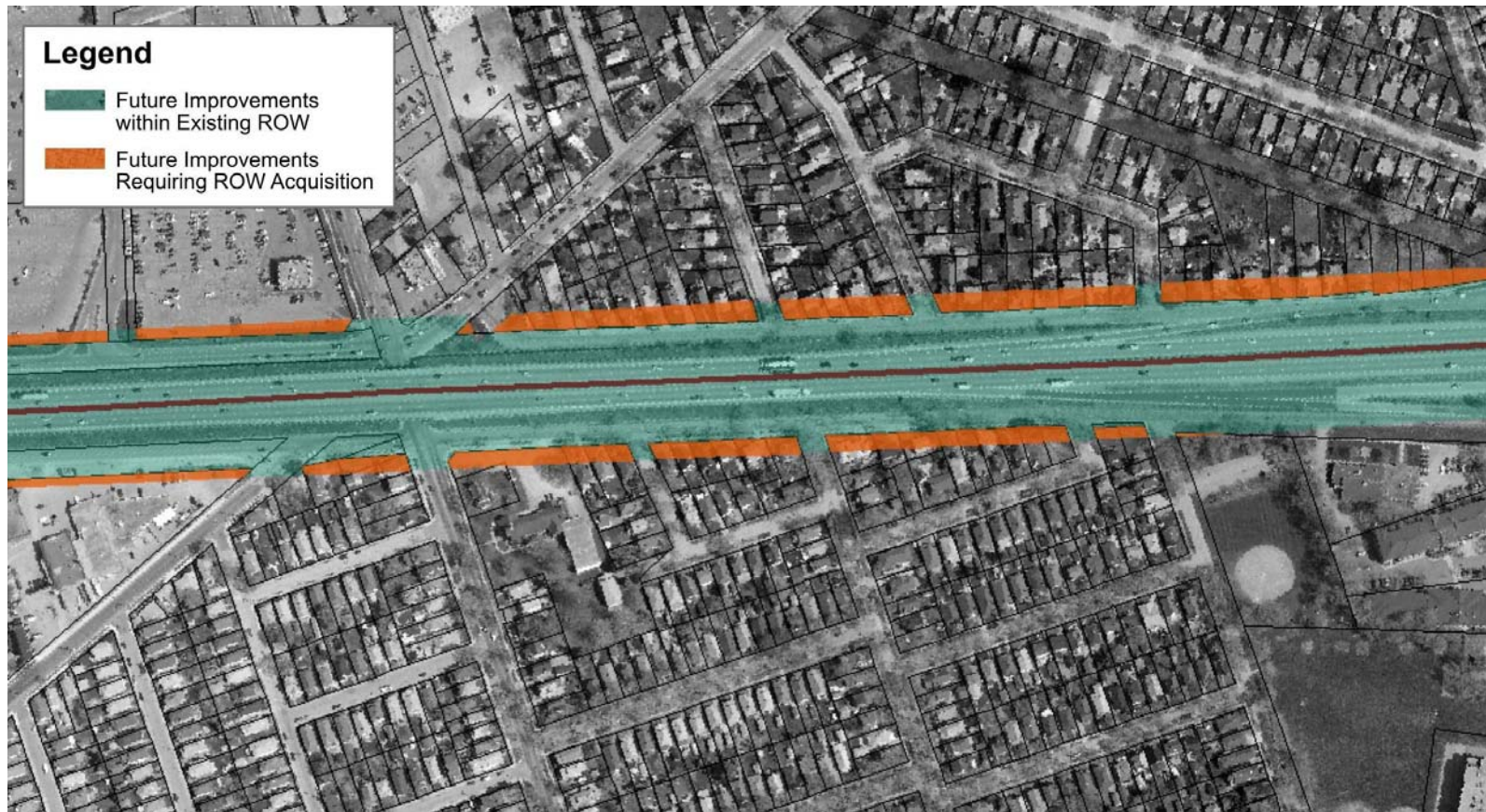
Exhibit 4-29: Sample Application of Mainline Widening Template
